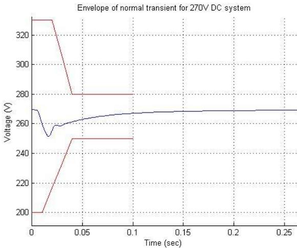
Figure 10. Voltage profile on healthy bus during fault with 21 mH inductor, for a 10 ms fault-clearing time.
