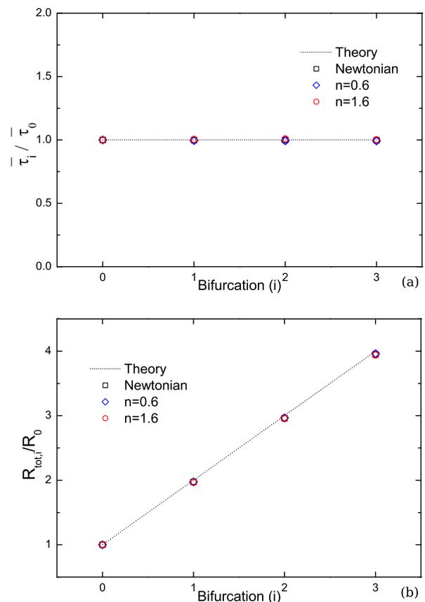
**Fig. 2.** Normalised wall shear-stress distribution (a) and flow resistance for various fluids (computed from Eq. (11)) (b) along the bifurcating network designed for a Newtonian fluid for  $\alpha_0 = 0.5$  and  $X = 1$  (Table 1).
