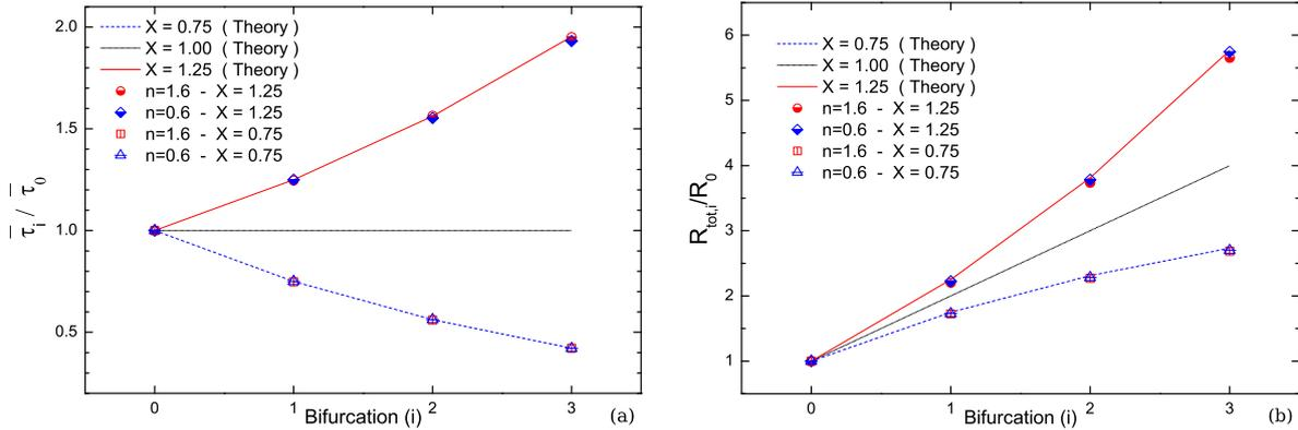
**Fig. 4.** Normalised wall shear-stress distribution (a) and flow resistance (computed from Eq. (11)) (b) along the customised bifurcating networks ( $\alpha_0 = 0.5$ ), designed using the biomimetic principle (Eq. 3) for  $n = 0.6$  and  $n = 1.6$  with  $X = 1.25$  and  $X = 0.75$ .
