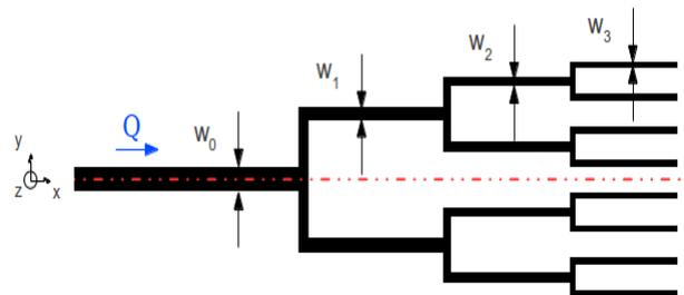
**Fig. 1.** Microfluidic bifurcating network of constant depth with 4 generations designed for a Newtonian fluid with an inlet aspect ratio  $\alpha_0 = 0.5$  and  $X = 1$ . The dashed-dotted line illustrates the symmetry conditions about  $y = 0$ .
