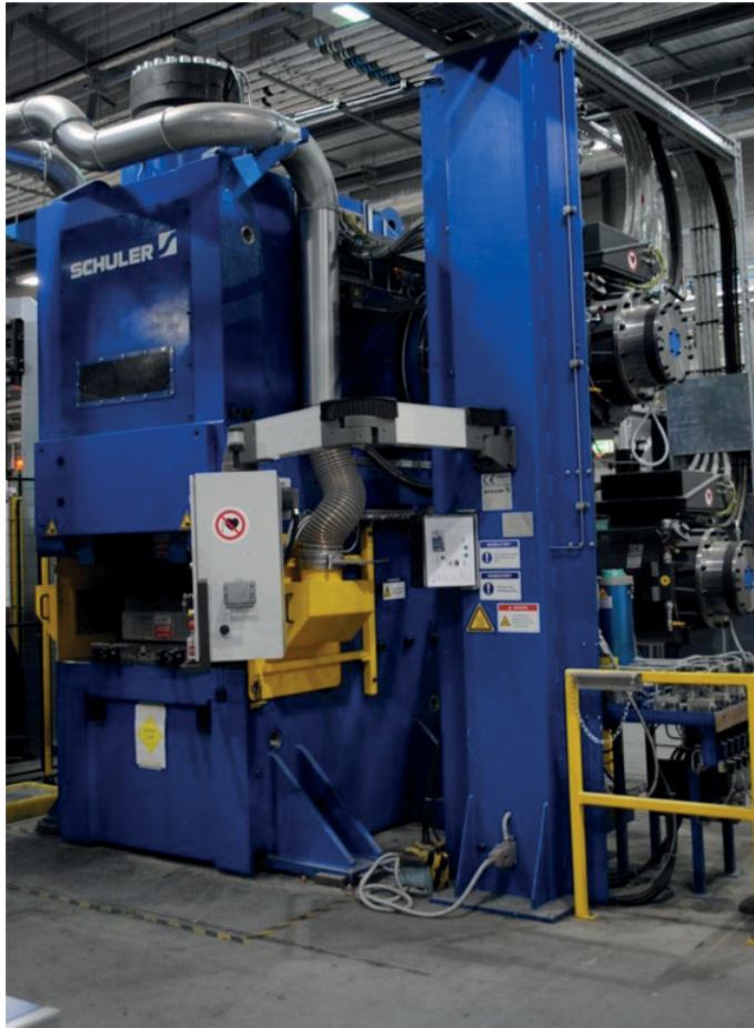
Figure 3. AFRC servo-driven multi-axis press. The motors are just visible on the right hand side of the press.
