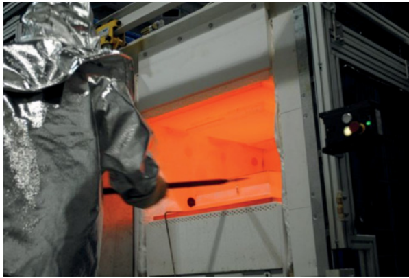
Figure 6. Removal of superplastically formed part from 200 tonne forming press. The forming cycle is developed using a finite element based approach to control the strain rate within the part to be within the optimum forming window.
