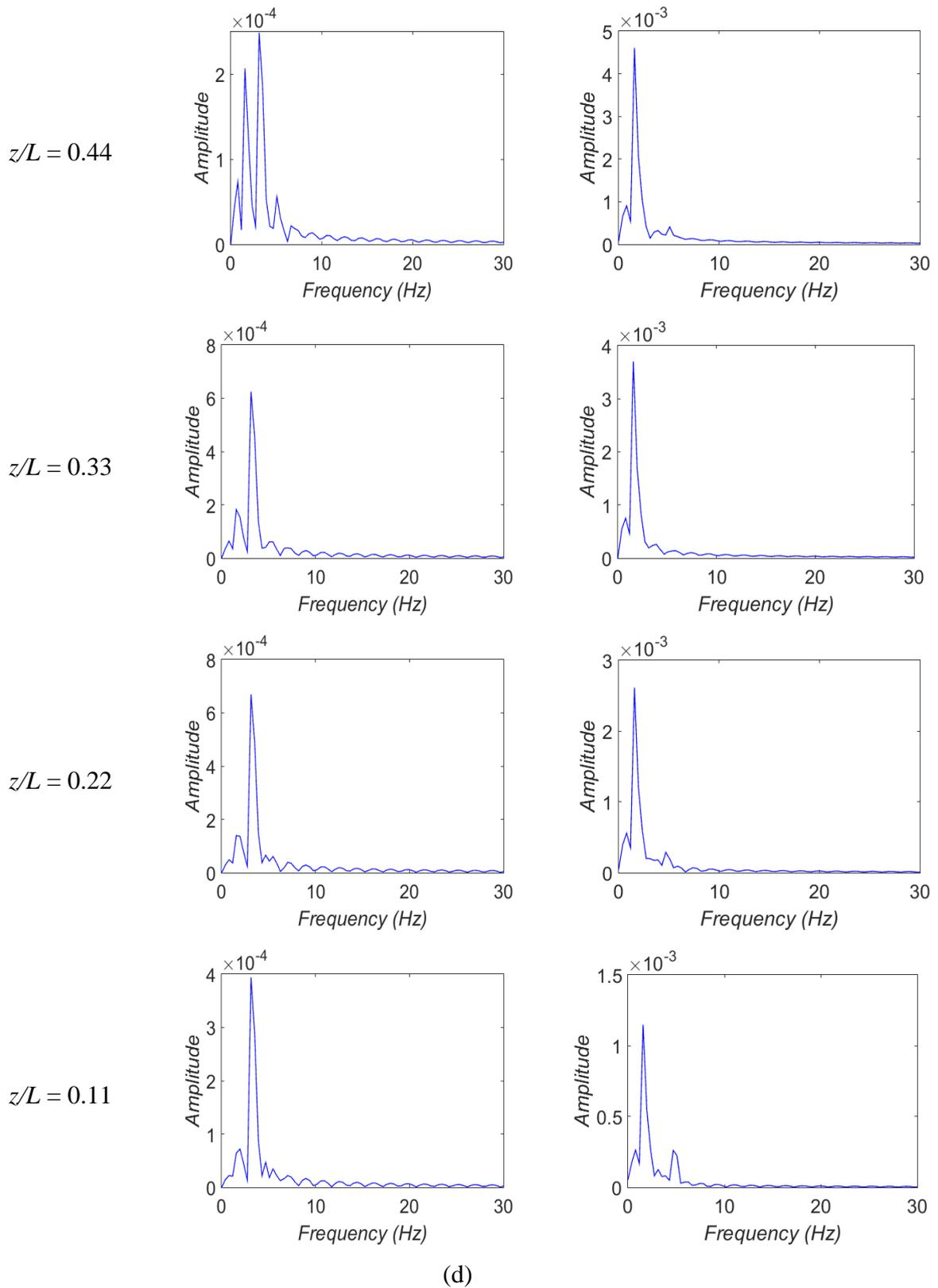
Fig. 11 Displacements and oscillation frequencies along the riser: (a) displacement time histories (# 1103), (b) oscillation frequencies (# 1103), (c) displacement time histories (# 1201) and (d) oscillation frequencies (#1201).
