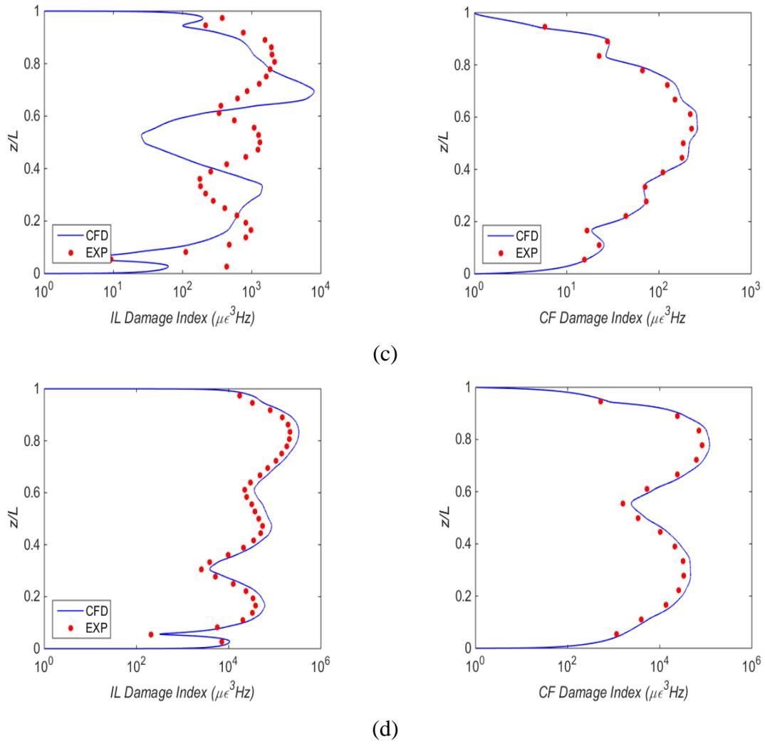
Fig. 14 Comparison of the fatigue damage indices: (a) # 1103, (b) # 1105, (c) # 1201 and (d) # 1205.
