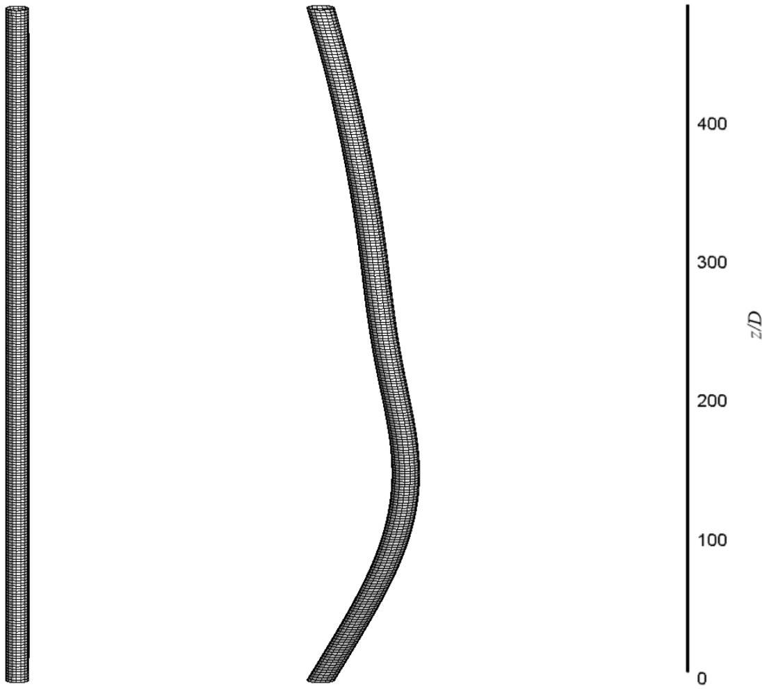
Fig. 4 FEA mesh: (a) initial mesh and (b) mesh with riser deflection.
