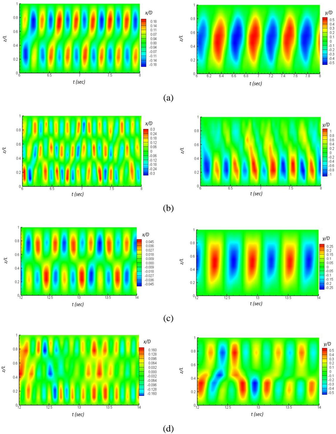
Fig. 7 The IL and CF motion evolution responses along the riser: (a) # 1103, (b) # 1105, (c) # 1201 and (d) # 1205.
