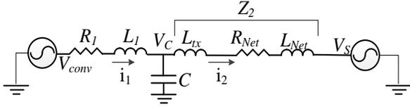
Figure 1. Schematic of VSC connected to power grid.
