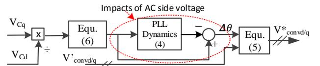
Figure 4. Simplified schematic of rotation because of PLL.
