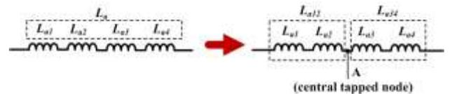
Fig. 2. Central-tapped winding of a 12/8 SRM.
