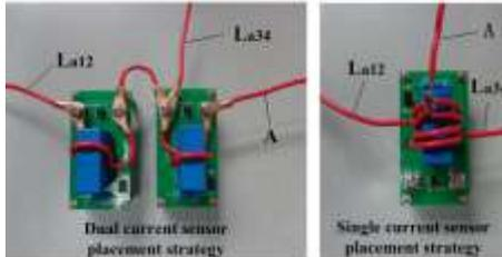
(b) Details of the two current sensors placement methods
