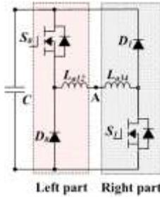
Fig. 3. Two parts of phase converter.
