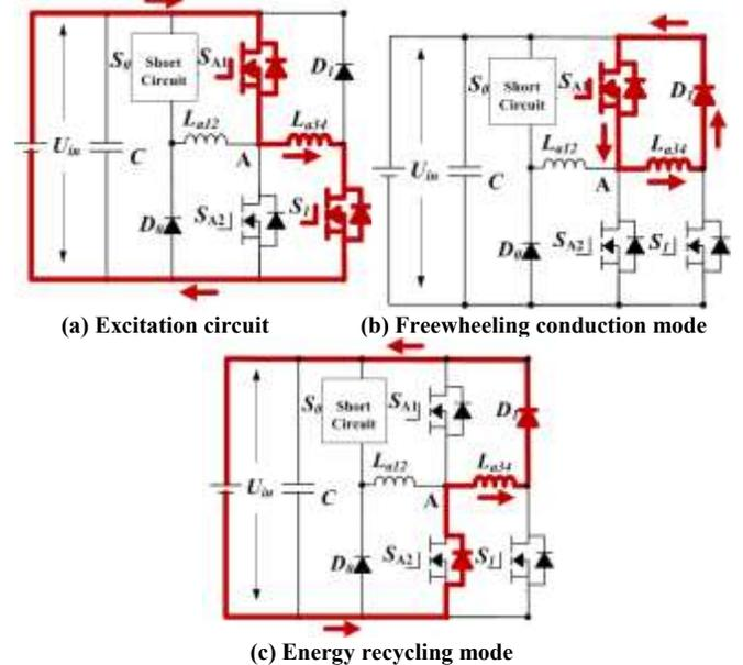
Fig. 8 Fault tolerance operation under  $S_0$  short circuit condition
