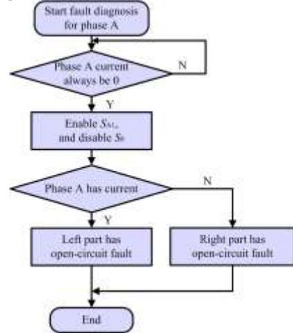
Fig. 5. Flowchart for the diagnosis of the open circuit fault.
