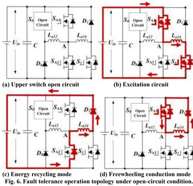
The same fault tolerance operation can be achieved, when  $D_0$  or  $L_{a12}$  is faulty. When the right part of one phase converter is under open-circuit fault condition, the left part of one phase converter and fault tolerance module can be combined to form a new fault tolerance topology, the same method as Fig. 6.
