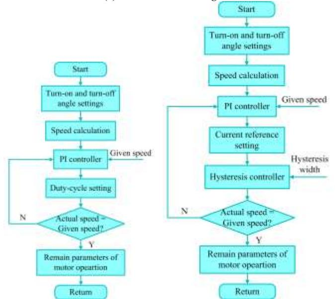
(b) Flowchart of algorithm for voltage-PWM control
