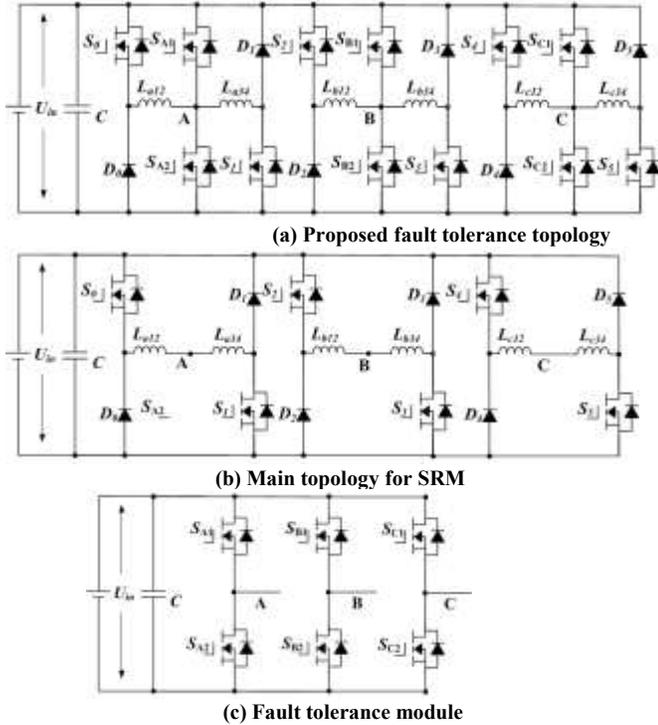
Fig. 4. Proposed topology for SRM fault tolerance operation.
