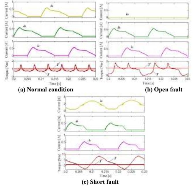
Fig. 16. Simulation results of voltage-PWM control mode under normal and fault conditions.
