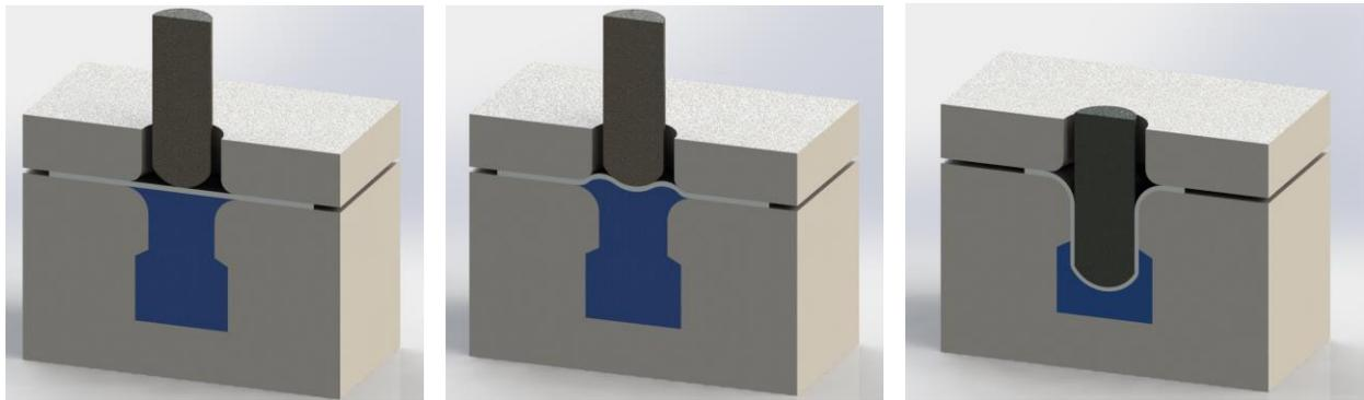
FIGURE 4. Schematic of pre-bulging in the opposite direction of the forming direction before hydroforming
