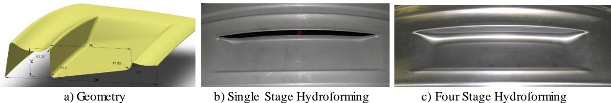
FIGURE 5. Multi-stage sheet hydroforming (Golovashchenko, et al., 2011)
