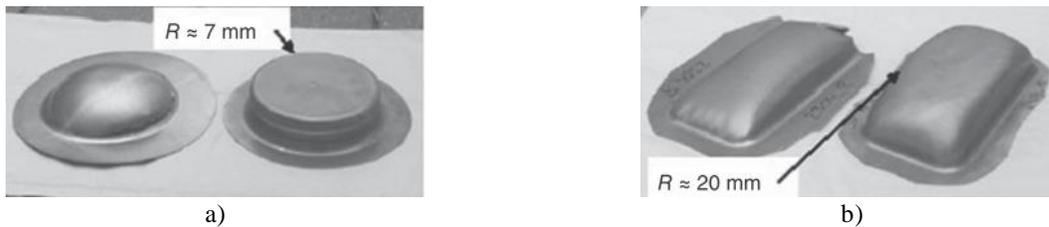
**FIGURE 8.** Normal vs. elevated temperature hydroforming operations of cups and rectangular sections (Koç, 2008)
