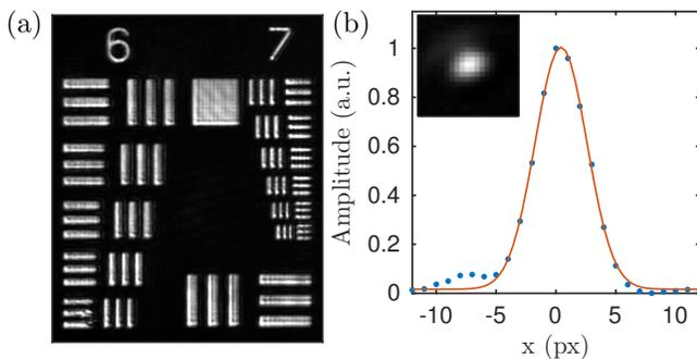
FIG. 4. (Color online). Calibration of imaging magnification and resolution for the ATOM objective using (a) 1951 USAF test card and (b) a  $5 \mu\text{m}$  pinhole. Camera pixels are  $8 \times 8 \mu\text{m}$ .
