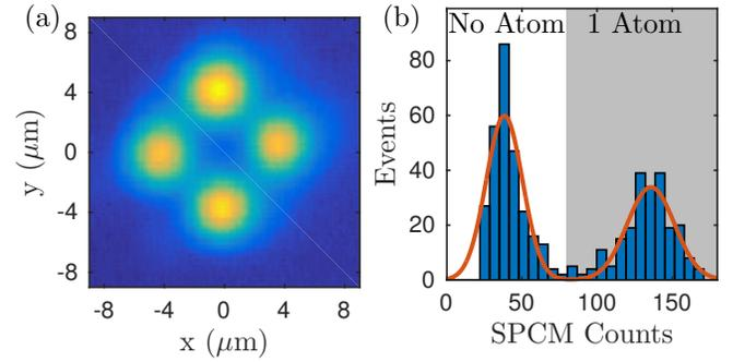
FIG. 5. (Color online). (a) Single-atom trap configuration using TRAP objective to create a single site GBA trap with four Gaussian spots with  $3 \mu\text{m}$  waist separated by  $6 \mu\text{m}$ . (b) Single atom fluorescence readout using the ATOM objective to demonstrate atom number discrimination, solid line shows fit to binomial distribution.
