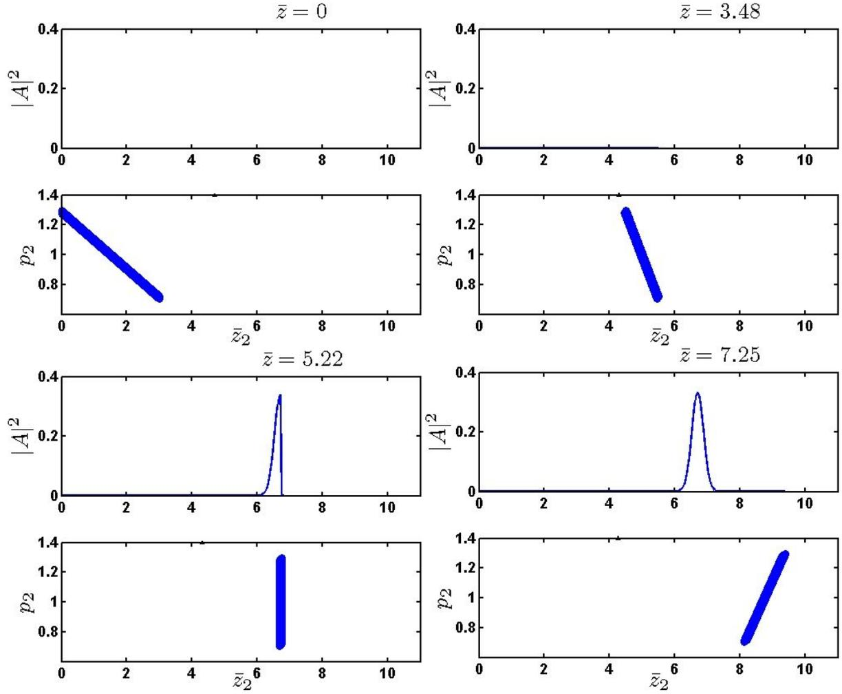
Figure 2: These 8 plots show the intensity and electron beam phase space at 4 different propagation distances. The initial chirp in the plot at  $\bar{z} = 0$  in the top left causes the electron pulse to compress and then decompress. When it is bunched to a length in  $\bar{z}_2$  of  $\lesssim 4\pi\rho$  (that is to say, less than a resonant radiation wavelength) it generates a single coherent spike in intensity.
