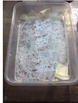
**Figure 2** Aggregates in silane solution
