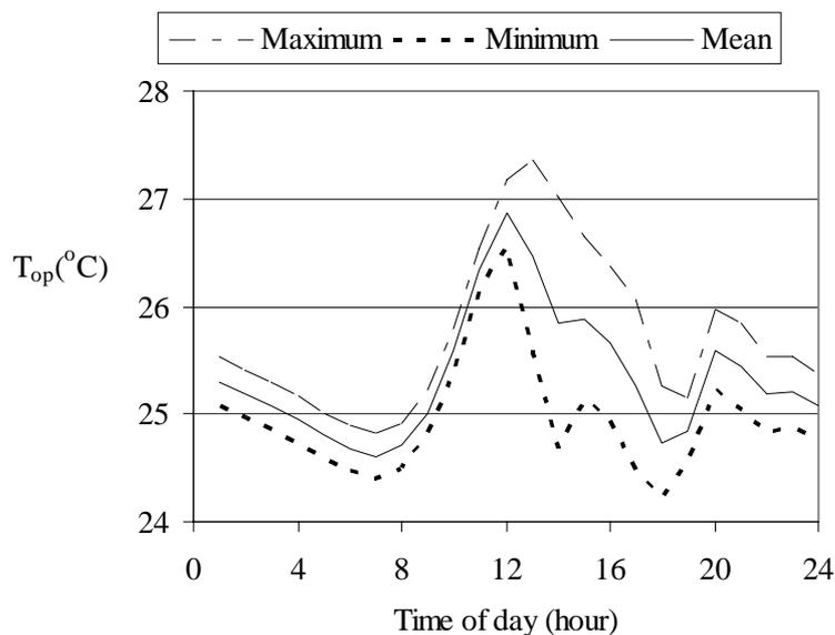
**Figure 7** The predicted range in operative temperature for a single day in summer day due to the variation in window opening behaviour represented by the stochastic nature of the Humphreys algorithm run in a Monte-Carlo mode.
