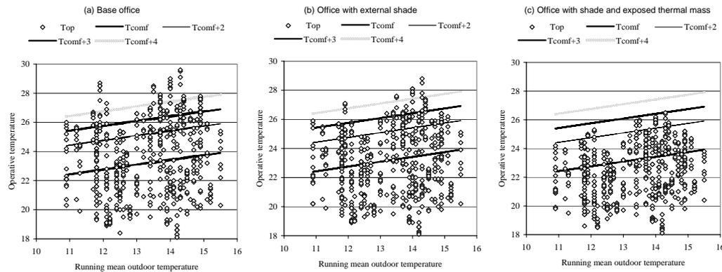
**Figure 6** The summer performance of the three office design variants is compared against the adaptive comfort criteria, the left graph (a) shows the baseline office, the center graph (b) shows the baseline office with an external shade added, the right graph (c) shows the baseline office with an external shade and an exposed concrete ceiling. All units are °C.
