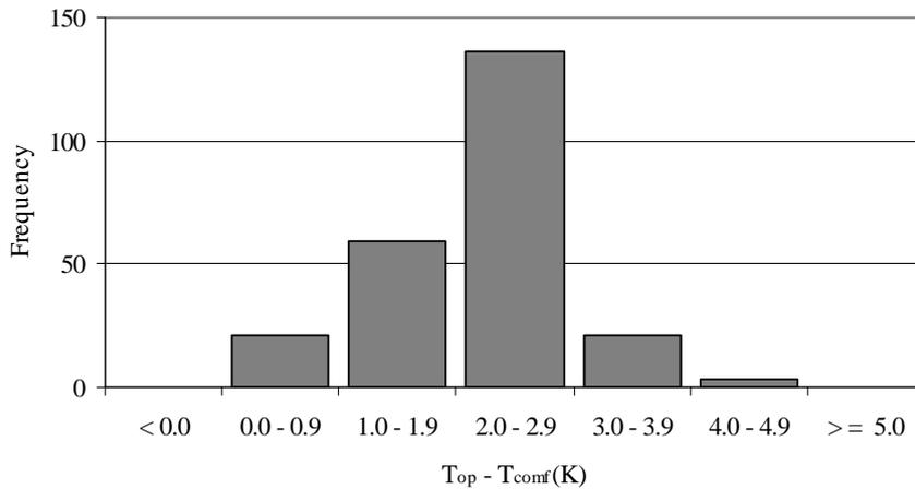
**Figure 8** The predicted distribution of the deviation from optimal thermal comfort temperature ( $T_{op} - T_{comf}$ ) for the same summer day as in Figure 10 due to the variation in occupant behaviour as embedded in the Humphreys algorithm.
