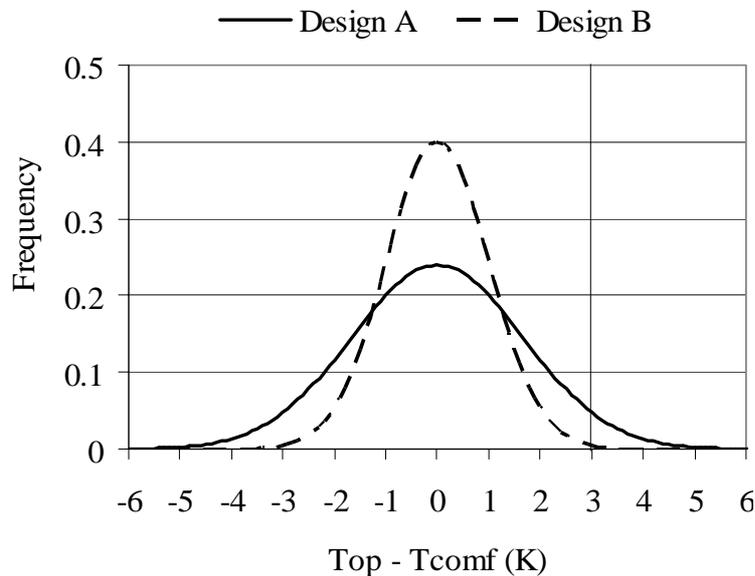
**Figure 10** Distributions representing the comfort performance of Design A and Design B for a range of input parameters representing variation in climate, internal gains, occupant behaviour, construction etc. Design A has a comfort capability of  $C = 1$  when compared to the  $T_{conf} + 3K$  limit for a category II building, Design B has a comfort capability of  $C = 0.6$ .
