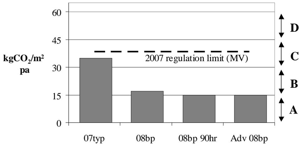
**Fig.3.** Carbon performance and energy rating for the mechanically ventilated (MV) design options with heat recovery (no cooling). Detailed input parameter values are given in appendix 1.
