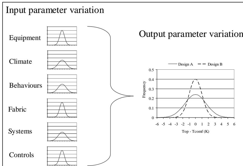
**Figure 9** The variation in input parameters combined in dynamic simulation using Monte-Carlo method to give a resulting variation in output parameters for Design A and Design B (see also Figure 10).
