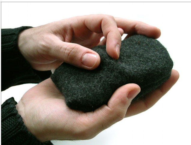
Figure 2: Prototype B: The input is the knob under the textile, the output is in the palm of the hand.
