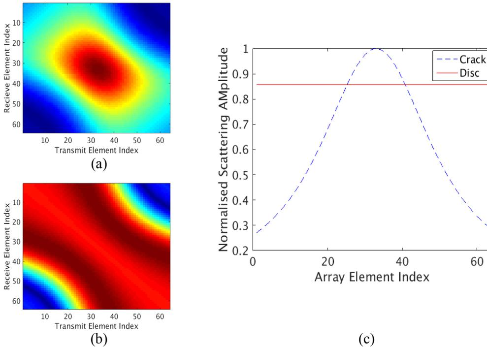
**Figure 3. Model scattering matrices (as calculated by the Born approximation) arising from (a) a 1.4mm crack and (b) a disc with diameter 1.4mm, both plotted at 3.1MHz. Plot (c) displays the corresponding pulse-echo responses.**
