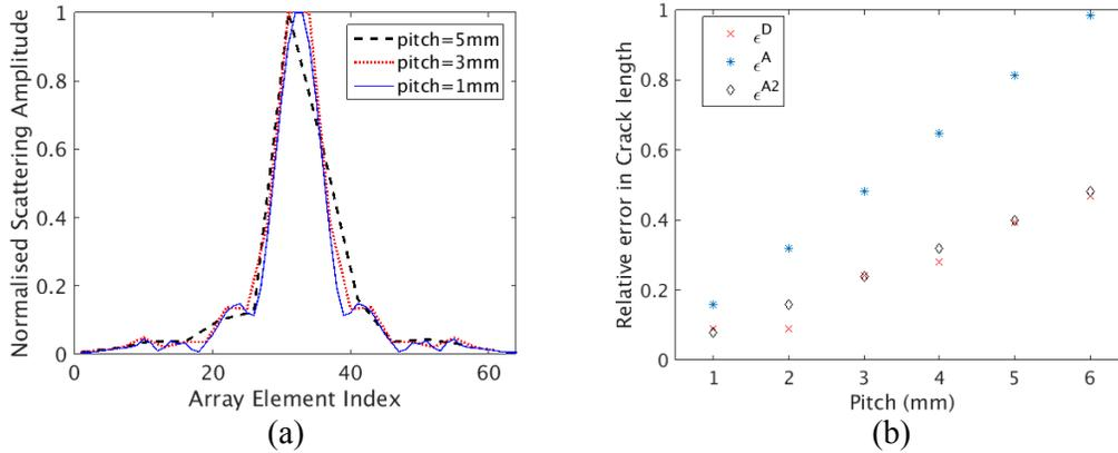
**Figure 4. (a) Plots of the pulse-echo response taken from subsets of the FMC data arising from dataset A, demonstrating the distortion caused by an increase in array pitch. (b) Plot of the analytically derived error assuming the approximated root is out by a pitch ( $\epsilon^A$ ) and half a pitch ( $\epsilon^{A/2}$ ). The actual error obtained via extraction of the roots from the pulse-echo is also plotted ( $\epsilon^D$ ).**
