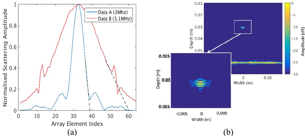
**Figure 2. (a) Pulse-echo responses from the scattering matrices arising from dataset A at 3MHz (blue line) and dataset B at 3.1MHz (red line). The dashed lines demonstrate how the root is estimated. (b) TFM image of the 1.4mm crack in dataset B.**
