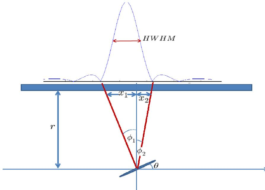
**Figure 1. Schematic demonstrating the relationship between the elements at which the roots of the pulse-echo response occur ( $x_1$  and  $x_2$ ), the depth  $r$  and the angles  $\phi_1$  and  $\phi_2$ .**
