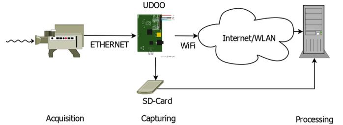
Fig. 1. Architecture of HSI system
