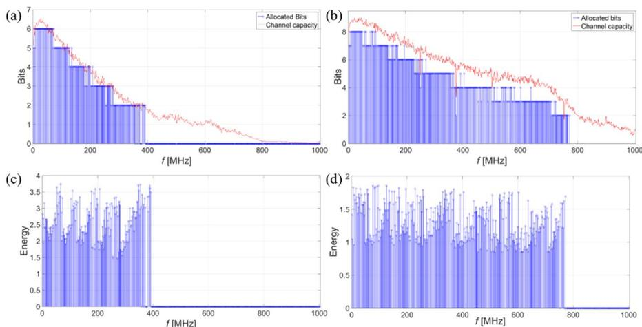
Figure 2 – allocated bits (a,b) and energy (c,d) for UV and violet  $\mu$ LEDs, respectively. The energy is normalized to the average energy in the OFDM frame.
