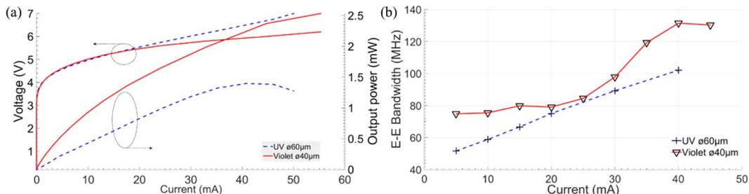
Figure 1 – (a) output power and voltage vs. current and (b) electrical -3dB bandwidth versus current for UV and violet  $\mu$ LEDs.
