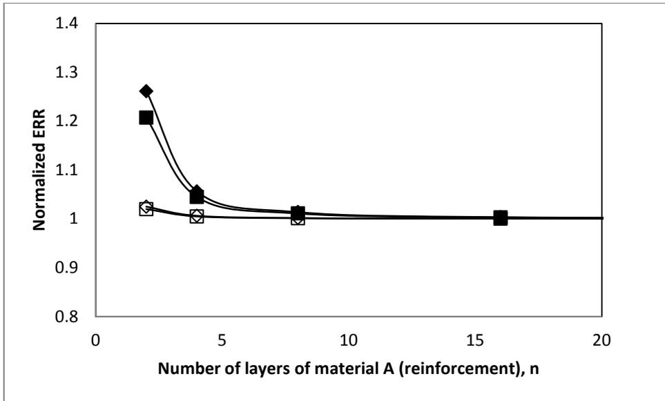
Figure 4 Unevenly loaded symmetric sample: variation in normalized mode I (squares) and mode II (diamonds) ERRs with number of layers of material A (reinforcement) for  $t_B = 0.1t_A$  (filled markers) and  $t_B = 0.01t_A$  (open markers)
