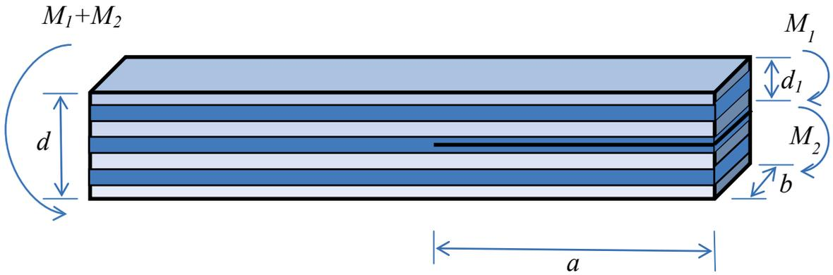
Figure 1 Composite laminate with delamination of length  $a$
