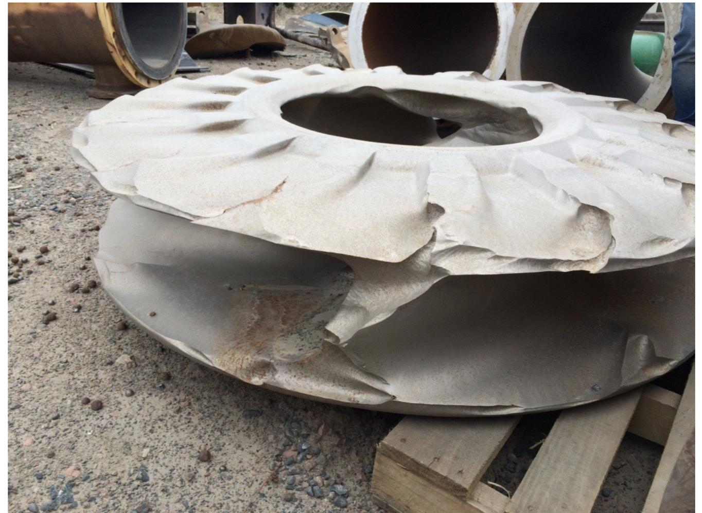
*Worn impeller of slurry pump*
