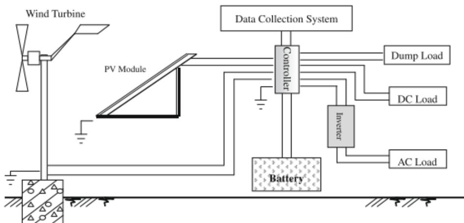
**Figure 1.** Block diagram of a hybrid solar-wind power generation system [5].
