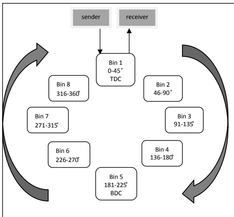
Figure 2: Schematic representation of wheel bins and crank angle sensor system.
