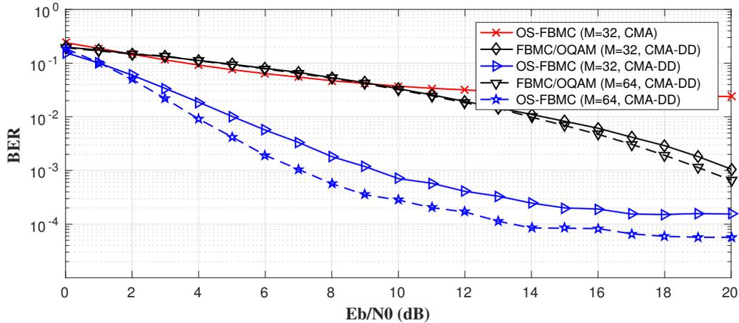
FIGURE 2. BER performances comparison of FBMC/OQAM to OS-FBMC
