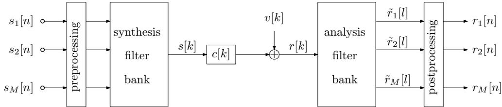
FIGURE 1. Block diagram of a general FBMC system.
