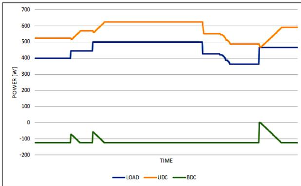
**Fig. 7.** UDC and BDC power response during a load change in the BDC buck mode.
