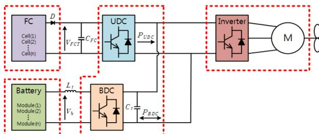
Fig. 1. Proposed hybrid power system for ships.
