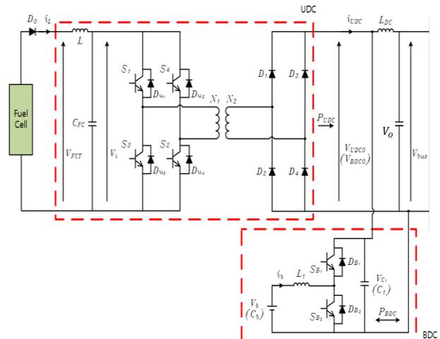
Fig. 2. Main circuit of power management system.
