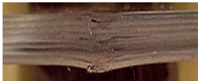
Fig. 13 Macro-photograph of the sectioned face of the [0/45/90]_{4s} composite plate.
