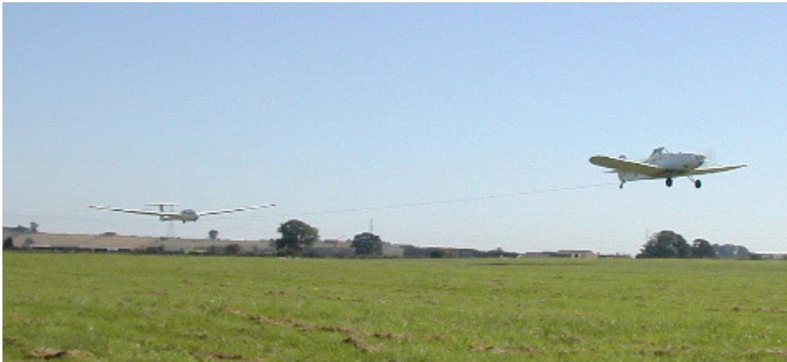
Figure 1: glider taking off on aero tow.
