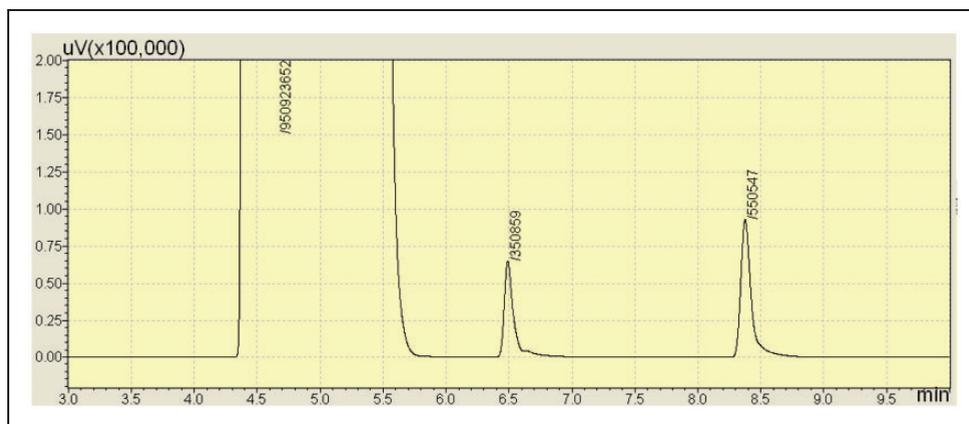
**Figure 4.** Gas chromatograph analysis of aqueous benzene, with toluene as internal standard and methanol as solvent. x-axis: time/min; y-axis: signal/ $\mu\text{V}$  k, where k is the magnification factor.
