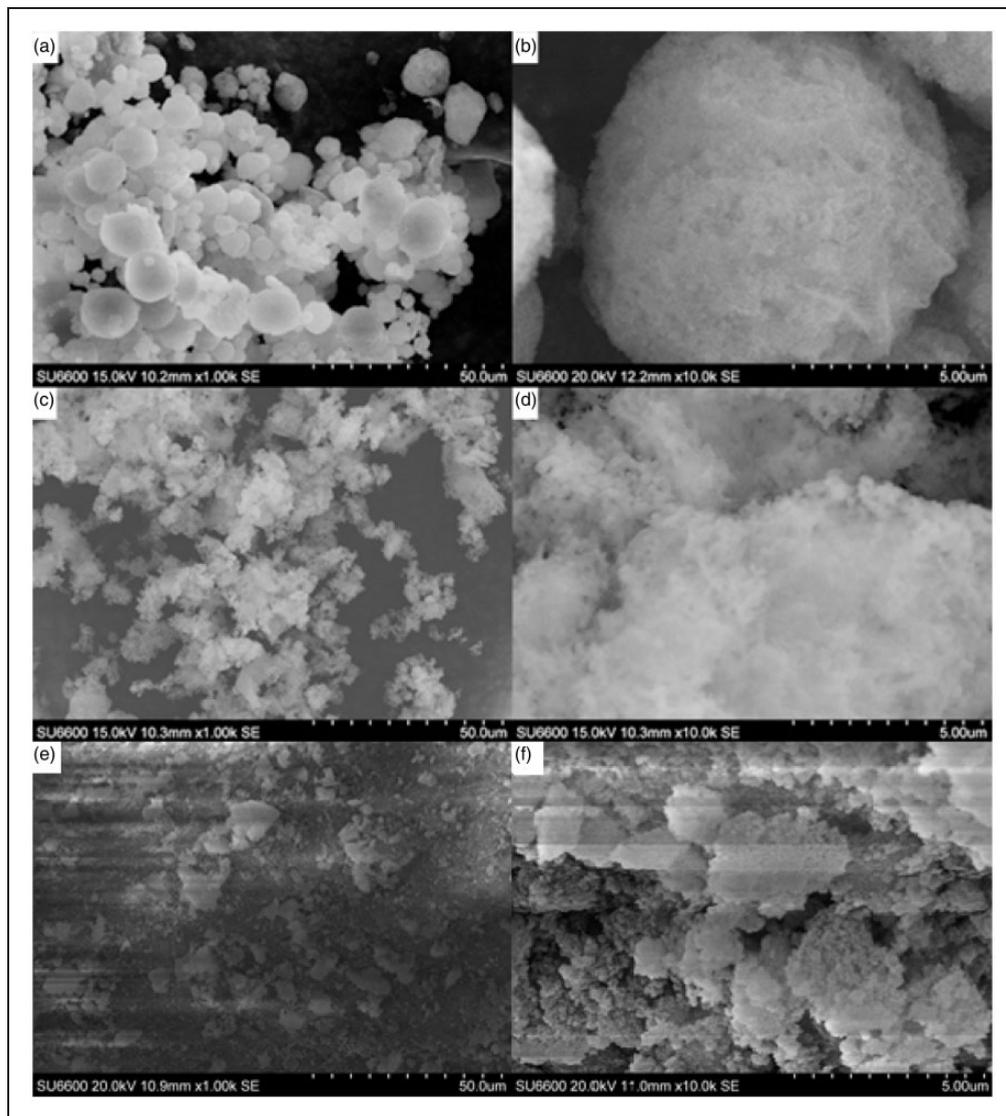
**Figure 1.** FE-SEM analysis of Quartzene samples: CMS (a:  $\times 1k$ , b:  $\times 10k$ ), ND (c:  $\times 1k$ , d:  $\times 10k$ ) and ZI (e:  $\times 1k$ , f:  $\times 10k$ ).
