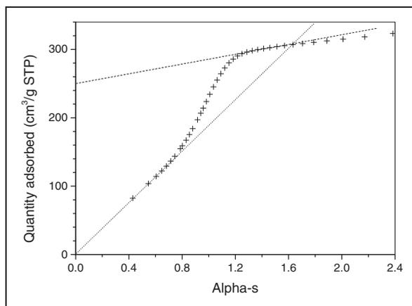
**Figure 3.**  $\alpha$ -plot analysis of ND nitrogen adsorption isotherm measured at 77 K (dotted line fit of low pressure data, dashed line fit of high pressure data).
