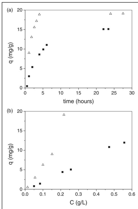
**Figure 7.** Kinetics (a) and isotherms (b) obtained for benzene adsorption by granular forms of Quartzene Z1 (filled squares) and Z1HPO (empty triangles) at 293 K.
