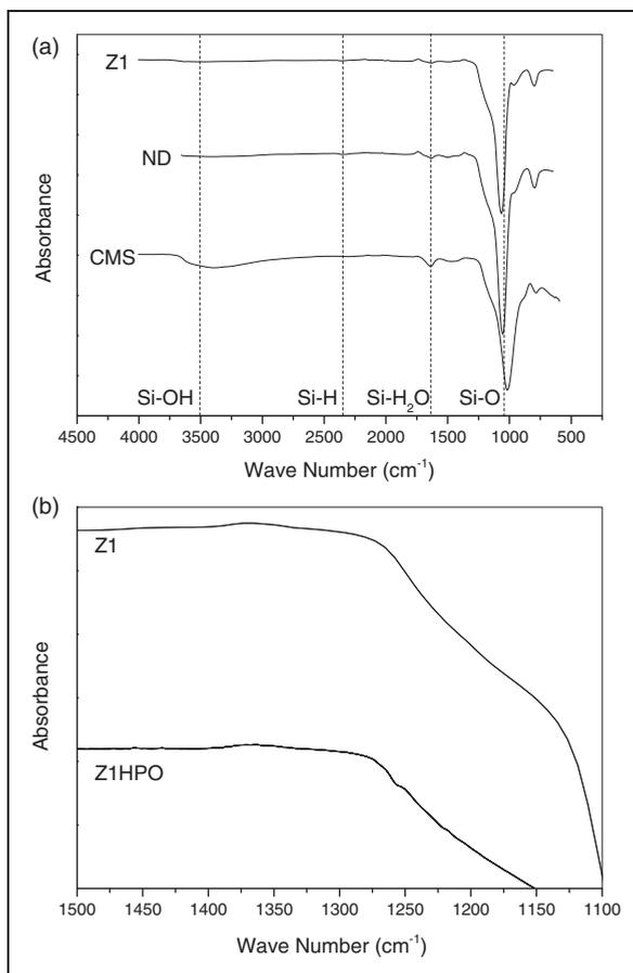
**Figure 2.** FT-IR spectra of silica samples: (a) Z1, ND and CMS and (b) comparison between the FT-IR spectra of Z1 and hydrophobic Z1HPO. The presence of Si-CH<sub>3</sub> bonds in the sample Z1HPO is confirmed by the small peak around 1250 cm<sup>-1</sup>.
