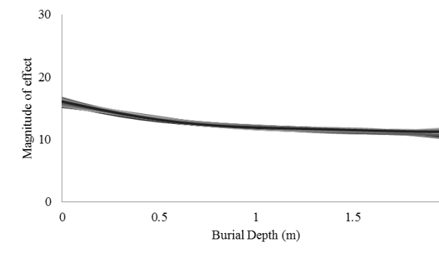
Figure 3c: Effect of Varying Soil Conductivity on Outlet Temperature
