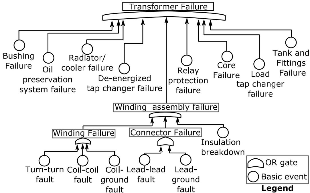
Figure 2. Simplified transformer Fault Tree model adapted from [3].
