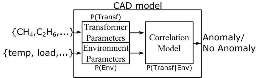
Figure 5. Conditional anomaly detection model.
