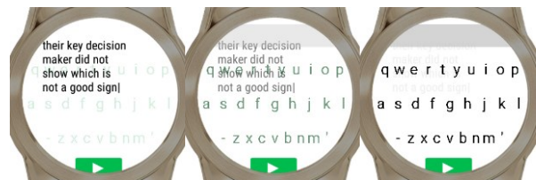
Figure 2: Experiment Tilt Controlled Layered Text Entry Interface – full text (left) through to full keyboard (right)
