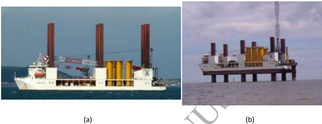
Figure 3: Jack-up installation vessel (a) in transit in jacked-down position (©Ross/CC-BY-SA-2.0) and (b) on-site in jacked-up position (©Ian Simons/CC-BY-SA-2.0)
