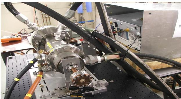
Fig. 1. A photo of the W-band gyro-TWA.
