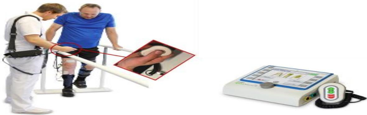
Fig.3: RehaMove system is used in gait rehabilitation therapy for patient with paraplegic. Reproduced with permission from HASOMED GmbH.
