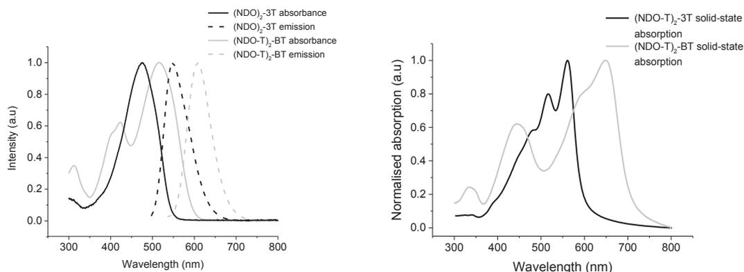
**Fig. 2.** UV/Vis absorption and emission spectra of  $10^{-5}$  M CH<sub>2</sub>Cl<sub>2</sub> solutions of **(NDO)<sub>2</sub>-3T** and **(NDO-T)<sub>2</sub>-BT** (left) and solid-state absorption spectra of **(NDO)<sub>2</sub>-3T** and **(NDO-T)<sub>2</sub>-BT** (right).
