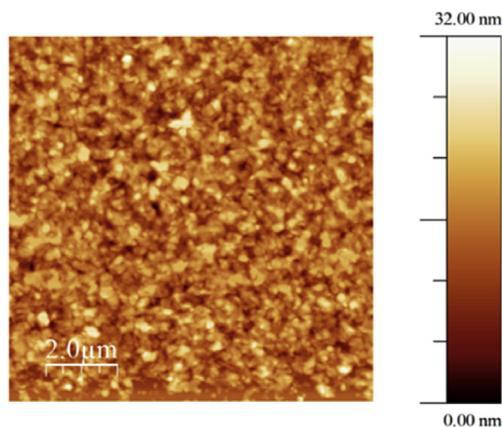
**Fig. 6.** AFM image of OFET fabricated using OTS SAM and (NDO-T)<sub>2</sub>-BT film cast from CHCl<sub>3</sub> solution with annealing at 120 °C. RMS roughness = 3.9 nm.
