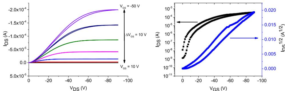
Fig. 5. Output (left) and transfer ( $V_{\text{DS}} = -50 \text{ V}$ ) (right) graphs of an OFET device containing  $(\text{NDO-T})_2\text{-BT}$ . SAM = OTS; solvent =  $\text{CHCl}_3$ ; annealed at  $120 \text{ }^{\circ}\text{C}$ . Channel length =  $5 \mu\text{m}$ ; channel width =  $1 \text{ cm}$ .
