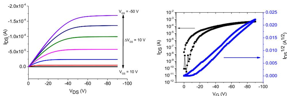
Fig. 4. Output (left) and transfer ( $V_{\text{DS}} = -50 \text{ V}$ ) (right) graphs of an OFET device containing  $(\text{NDO-T})_2\text{-BT}$ . SAM = OTS; solvent =  $\text{CHCl}_3$ ; unannealed. Channel length =  $20 \mu\text{m}$ ; channel width =  $1 \text{ cm}$ .
