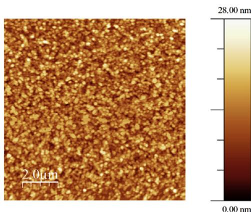
**Fig. 7.** AFM image of OFET fabricated using OTS SAMs and film cast from CHCl<sub>3</sub> solution without annealing. RMS roughness = 3.4 nm.
