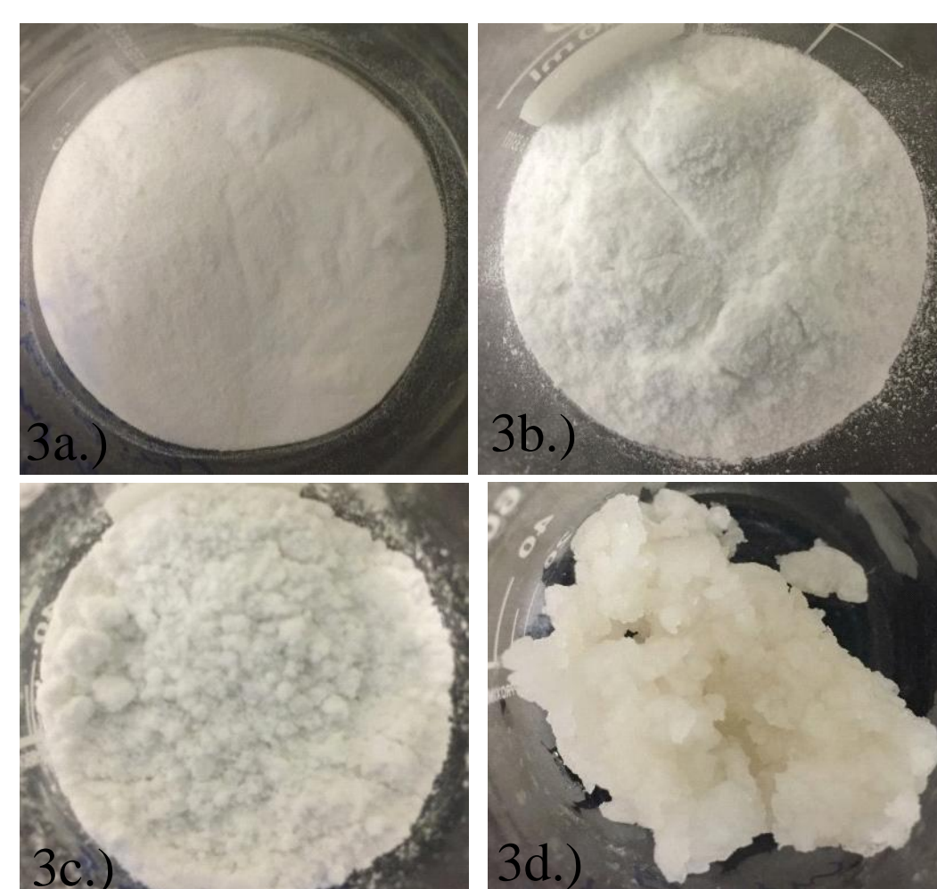
Figure 4: SEDDS loaded Syloid XDP 3150 manufactured with two kneading zones.
