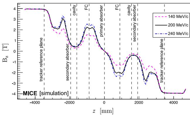
FIG. 5. Magnetic field  $B_z$  on-axis versus the longitudinal coordinate  $z$  for the cooling-demonstration lattice design for 200 MeV/c (solid black line), 140 MeV/c (dashed purple line), and 240 MeV/c (dot-dashed blue line) settings. The vertical dashed lines with labels show the positions of the tracker reference planes and the centres of the absorbers, rf cavities, and focus coil modules.
