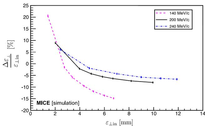
FIG. 10. Fractional change in emittance versus initial emittance ( $\epsilon_{\perp, \text{in}}$ ) for the cooling-demonstration lattice design measured at the tracker reference planes. The fractional change in emittance of the 140 MeV/c, 200 MeV/c, and 240 MeV/c lattices are shown as the purple-dashed, solid black, and dot-dashed blue lines, respectively. The error bars indicate the statistical precision that would be achieved using a sample of 100,000 muons.
