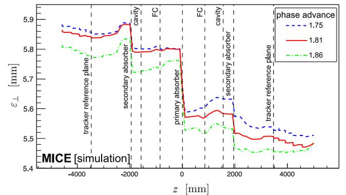
FIG. 4. 4D emittance evolution in the cooling-demonstration lattice for 200 MeV/ $c$  settings with a phase advance of  $2\pi \times 1.75$  (dashed blue line),  $2\pi \times 1.81$  (solid red line) and  $2\pi \times 1.86$  (dot-dashed green line). The vertical dashed lines with labels show the positions of the tracker reference planes and the centers of the absorbers, rf cavities, and focus coil modules.
