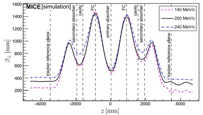
FIG. 6.  $\beta_{\perp}$  versus the longitudinal coordinate  $z$  for 200 MeV/c (solid black line), 140 MeV/c (dashed purple line) and 240 MeV/c (dot-dashed blue line) in the cooling-demonstration lattice. The vertical dashed lines with labels show the positions of the tracker reference planes and the centers of the absorbers, rf cavities, and focus coil modules.
