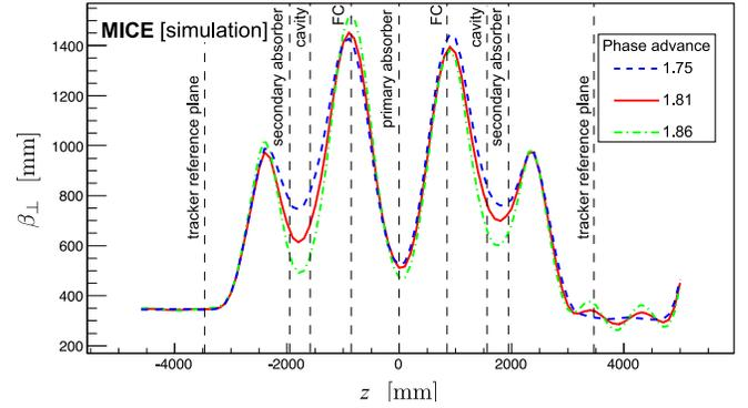
FIG. 3. Transverse 4D beta-function versus longitudinal coordinate  $z$  in the cooling-demonstration lattice for 200 MeV/ $c$  settings with a phase advance of  $2\pi \times 1.75$  (dashed blue line),  $2\pi \times 1.81$  (solid red line) and  $2\pi \times 1.86$  (dot-dashed green line). The vertical dashed lines with labels show the positions of the tracker reference planes and the centers of the absorbers, rf cavities, and focus coil modules.
