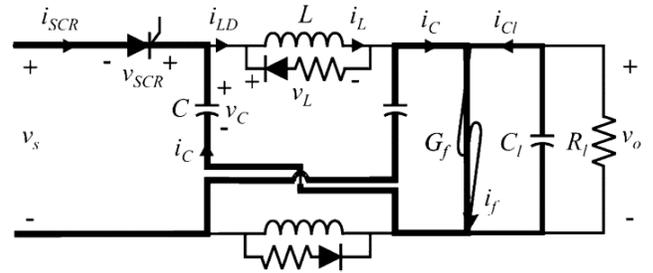
Fig. 8. Structure of a z-source breaker
