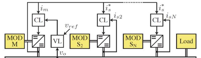
Fig. 5. Master-Slave (MS) control of a DC microgrid
