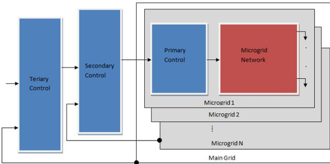
Fig. 3. Hierarchal control of a DC microgrid
