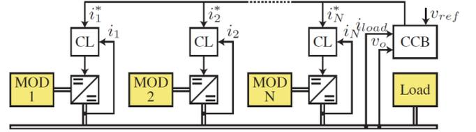
Fig. 4. Centralized control of a DC microgrid
