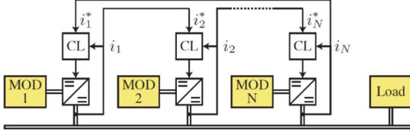
Fig. 6. Circular chain control of a DC microgrid
