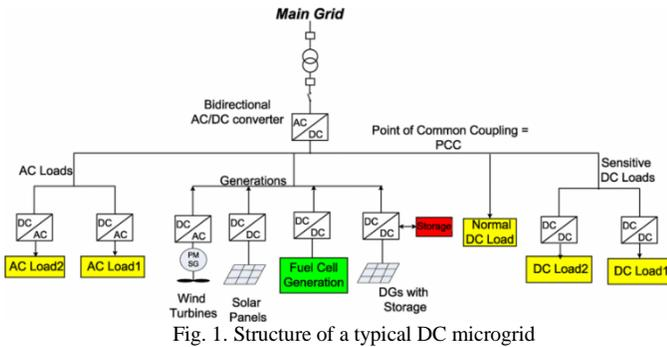
Fig. 1. Structure of a typical DC microgrid
