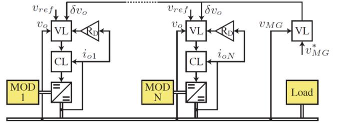
Fig. 7. Droop control of a DC microgrid via virtual output impedance
