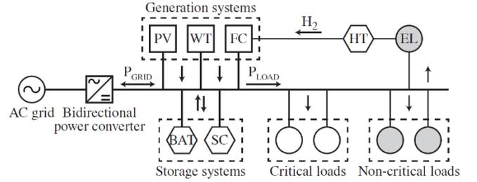
Fig. 2. Power flow in a DC microgrid
