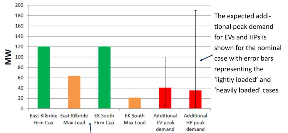
For comparison, the firm capacity and current maximum load of the two Grid Supply Points (GSPs) serving East Kilbride – East Kilbride and East Kilbride South—are shown [12].
