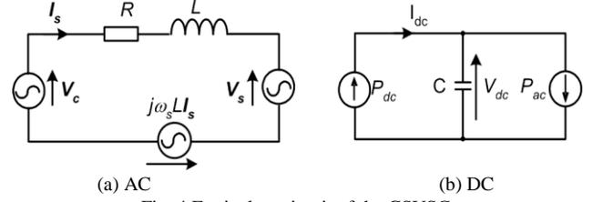
Fig. 4 Equivalent circuit of the GSVSC
