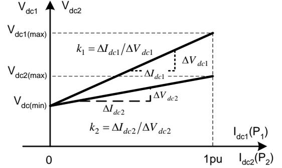
Fig. 3 DC droop characteristics for GSVSC1 and GSVSC2
