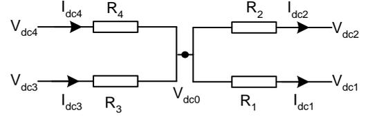
Fig. 2 Steady-state DC equivalent circuit of the four-terminal system
