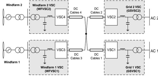
Fig. 1 Single-line diagram of wind farm integration using a MT VSC HVDC system.
