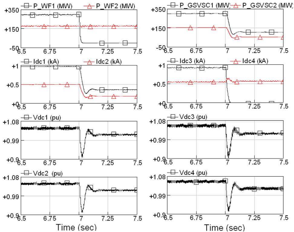
Fig. 8 Simulation results during the disconnection of WF1 with the loss of 300MW infeed power at 7s.
