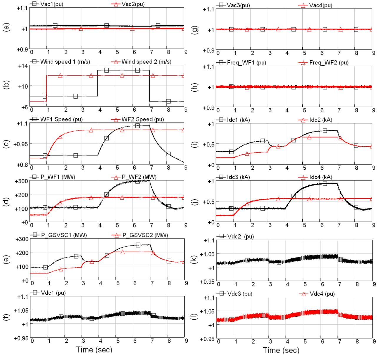
Fig. 7 Simulation results with variation of wind speed: (a) Onshore grid AC voltage; (b) Wind speed; (c) DFIG rotor speed; (d) Power generated by the wind farms; (e) GSVSC1 DC voltage; (f) Power transmitted by the two GSVSCs; (g) Offshore AC voltage; (h) Offshore AC frequency; (i) GSVSC DC current; (j) WFVSC DC current; (k) GSVSC2 DC voltage; (l) WFVSC DC voltage.
