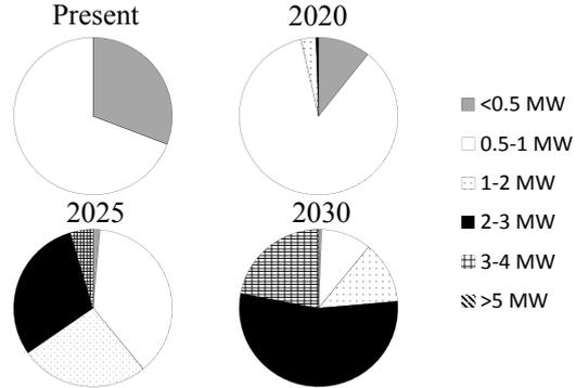
Figure 3: Distribution of turbine capacity reaching its 20th year of operation [5]. Boundary turbines are categorised in the higher class.
