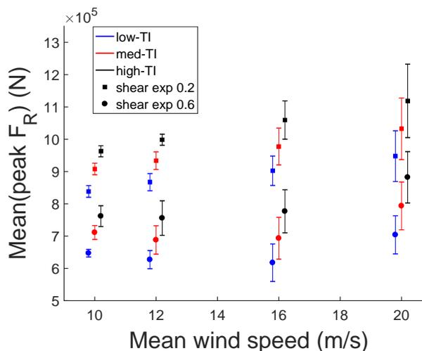
**Figure 6.** Mean peak radial loading over each set of six wind fields with parameters in common. Note, results have been staggered about each mean wind speed for clarity.
