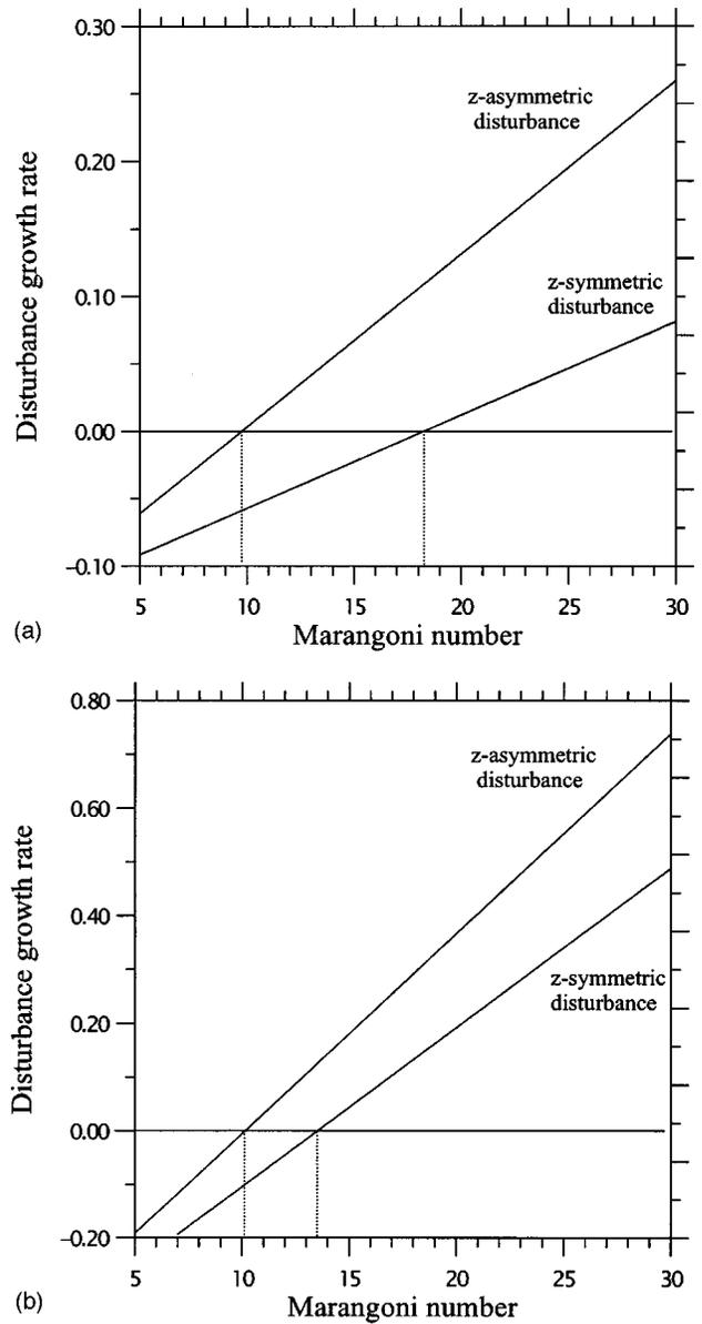
FIG. 18. Growth rates as function of the Marangoni number and determination of the first critical Marangoni number (mirror-symmetric and anti-symmetric disturbances): (a)  $A_F = 0.5$ , (b)  $A_F = 1.5$ .
