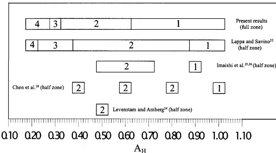
FIG. 17. Comparison between the azimuthal wave number of the full-zone configuration (present results) and available results dealing with the half zone configuration ( $Pr=0.01$ ).
