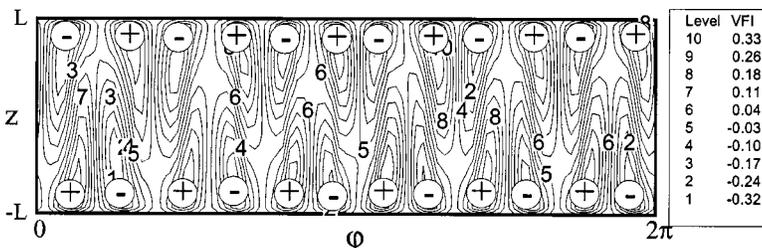
FIG. 14. Surface azimuthal velocity distribution at the 3D stationary state ( $A_F=0.3$ ,  $m=6$ ,  $Ma \approx 30$ ,  $\Phi=12.3$  [w]).
