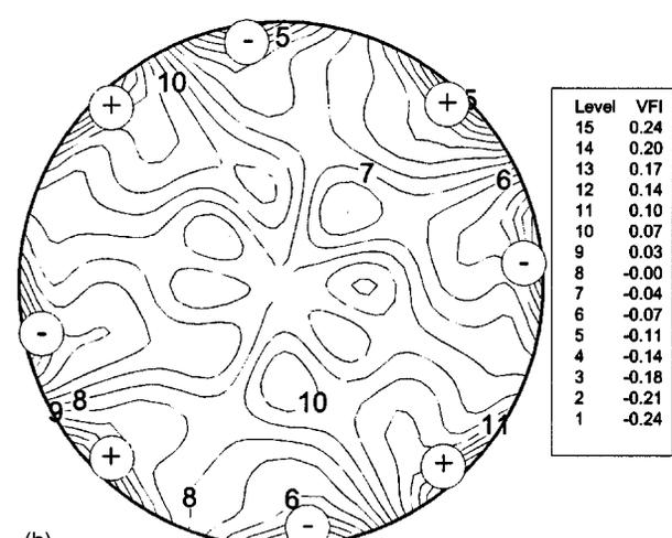
FIG. 9. Structure of 3D Marangoni flow with  $m=2$ ,  $A_F=0.8$ ,  $Ma\approx 30$ ,  $\Phi=4.57$  [w]: (a), (b) axial velocity in the cross-sections  $z=0.5$ ,  $z=0$ .
