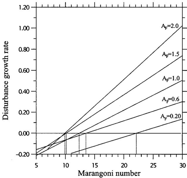
FIG. 15. Growth rates as function of the Marangoni number and determination of the first critical Marangoni number for different values of the aspect ratio.
