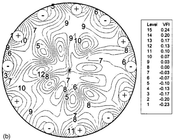
FIG. 12. Structure of 3D Marangoni flow with  $m=3$ ,  $A_F=0.6$ ,  $Ma \approx 30$ ,  $\Phi=6.27$  [w]: (a), (b), axial velocity in the cross-sections  $z=0.5$ ,  $z=0$ .
