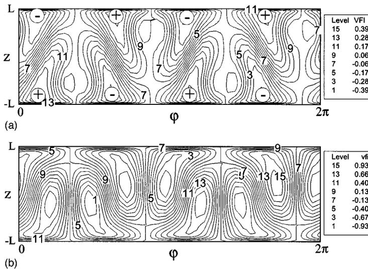
FIG. 7. (a) Surface azimuthal velocity distribution ( $A_F=0.8$ ,  $m=2$ ,  $Ma\approx 30$ ,  $\Phi=4.57$  [w], numerical results); (b) plot of the analytical expansion of the surface azimuthal velocity:  $[\tilde{F}_1(z)\sin(m\varphi+G_o)-\tilde{F}_2(z)\sin(Nm\varphi+NG_o)]$ ,  $\tilde{F}_1(z)=z(1-z^{20})^2$ ,  $\tilde{F}_2(z)=(1-z^2)^2$ ,  $m=2$ ,  $N=2$ ,  $G_o=1$ .
