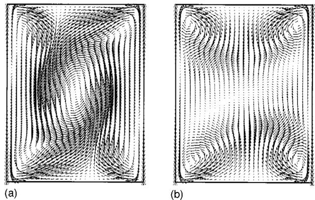
FIG. 4. Velocity field in the meridian plane ( $A_F=1.3$ ,  $Ma\approx 30$ ,  $\Phi=2.54$  [w],  $m=1$ ); (a)  $\varphi \approx 3\pi/4$ , (b)  $\varphi \approx 5\pi/4$ .
