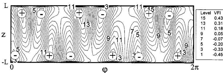
FIG. 11. Surface azimuthal velocity distribution at the 3D stationary state ( $A_F=0.6$ ,  $m=3$ ,  $Ma\approx 30$ ,  $\Phi=6.27$  [w]).
