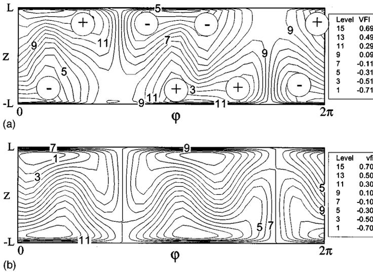
FIG. 3. (a) Surface azimuthal velocity distribution at the 3D stationary state ( $A_F=1.3$ ,  $m=1$ ,  $Ma\approx 30$ ,  $\Phi=2.54$  [w], numerical results); (b) plot of the analytical expansion of the surface azimuthal velocity:  $[\tilde{F}_1(z) \sin(m\varphi+G_0) - \tilde{F}_2(z) \sin(Nm\varphi+NG_0)]$ ,  $\tilde{F}_1(z) = z(1-z^{20})^2$ ,  $\tilde{F}_2(z) = 0.3(1-z^2)^2$ ,  $m=1$ ,  $N=4$ ,  $G_0=1$ .
