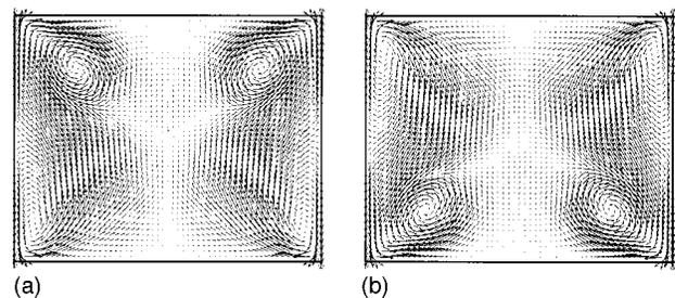
FIG. 8. Velocity field in the meridian plane ( $A_F=0.8$ ,  $Ma\approx 30$ ,  $\Phi=4.57$  [w],  $m=2$ ); (a)  $\varphi\approx\pi/2$ , (b)  $\varphi\approx\pi$ .
