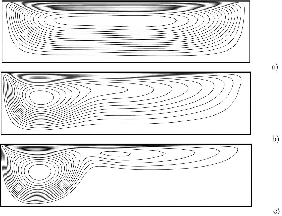
**Figs. 2:** Structure of pure Marangoni convection for  $\text{Pr}=0.01$  (Silicon) and open cavity with aspect ratio  $A=4$  (cold and hot sides on the left and on the right of each frame respectively, upper and lower boundaries with adiabatic conditions): (a)  $\text{Ma}=10$ , (b)  $\text{Ma}=100$ , (c)  $\text{Ma}=1000$  ( $\text{Ma}$  based on the width of the cavity).
