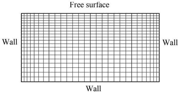
Fig. 4: Example of grid for the open cavity problem obtained combining one-dimensional stretching function along  $x$  and  $y$  ( $\phi=2$  and  $Q=1$ ).
