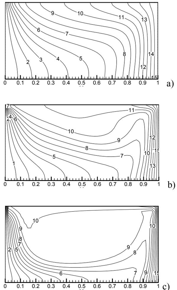
**Figs. 3:** Open cavity problem,  $Pr=15$ ,  $A=2.0$ , temperature distribution, cold wall on the left side, hot wall on the right side, upper and lower boundaries with adiabatic conditions: (a)  $Ma=10^3$ , (b)  $Ma=10^4$ , (c)  $Ma=10^5$ . (level 1  $\rightarrow T=0.06$ , level 15  $\rightarrow T=0.94$ ;  $\Delta level=0.06$ )
