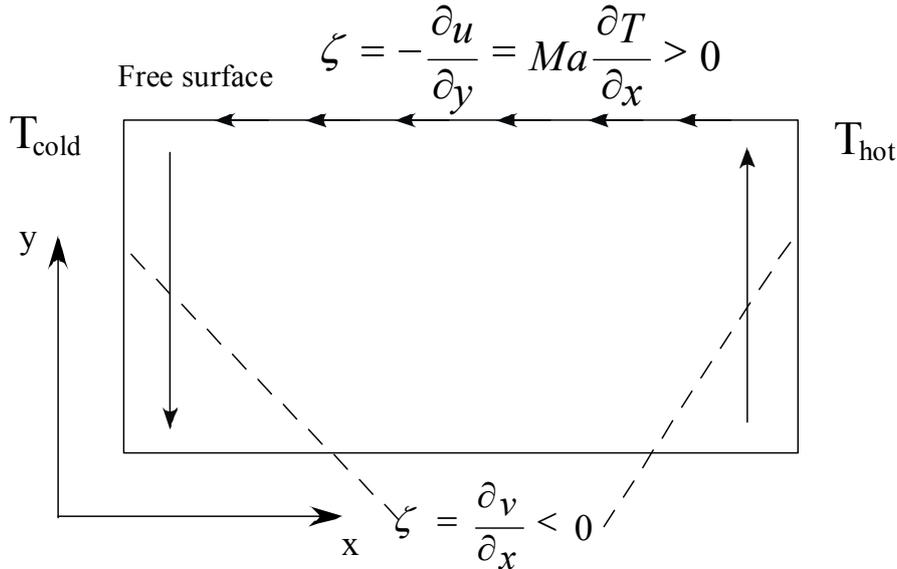
Fig. 5: Sketch of the conditions responsible for the viscous singularities ( $u$  and  $v$  are the velocity components along  $x$  and  $y$  respectively).
