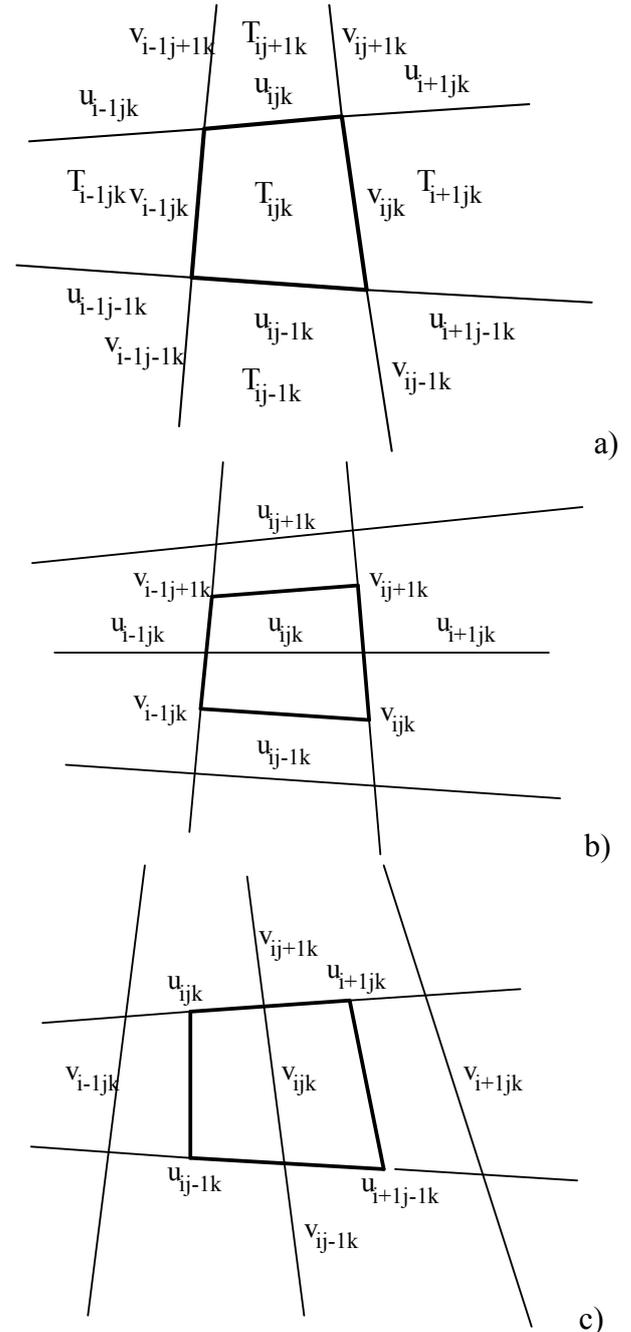
**Figs. 1:** Staggering for the different variables: the figures show the collocation of temperature and velocity components in the x-y plane (u and v are the velocity components along x and y respectively, the i and j subscripts indicate the relative position along x and y of the nodal values).
