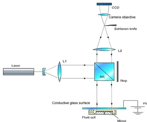
**Figure 6** – Sketch of the Shlieren/shadowgraphy setup available in FSL. The Shlieren knife can be removed to perform shadowgraphy. The Fluid cell sketched in the drawing is that of the previous figure.
