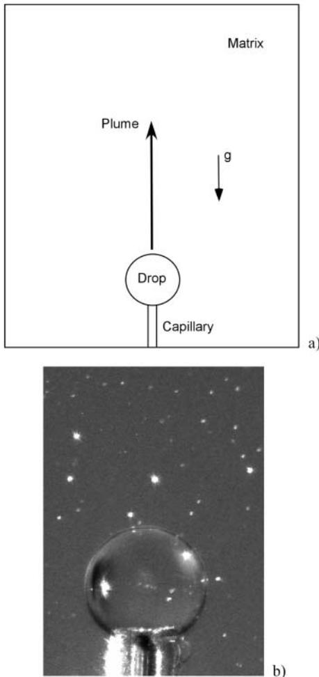
**Figure 1** (a) Sketch of the geometrical configuration; (b) liquid drop at the tip of the capillary tube.
