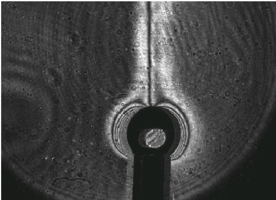
Figure 4. Rising plume from a droplet of Methanol dissolving in Cyclohexane at ambient temperature (initial drop volume of  $3 \mu\text{l}$ )
