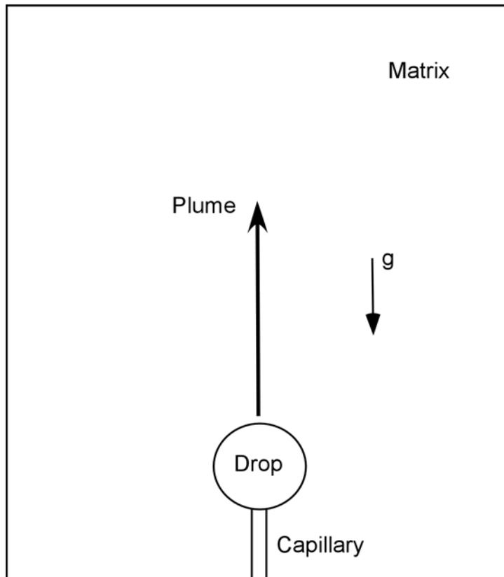
Figure 1: Sketch of the geometrical configuration
