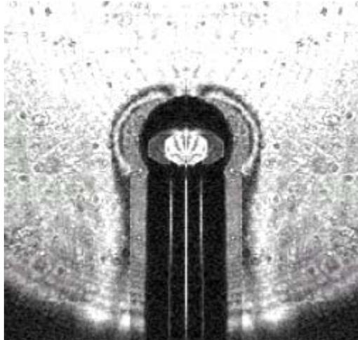
Figure 3. Descending flow from a droplet of Methanol dissolving in Hexane at ambient temperature (initial drop volume of  $1.5 \mu\text{l}$ )
