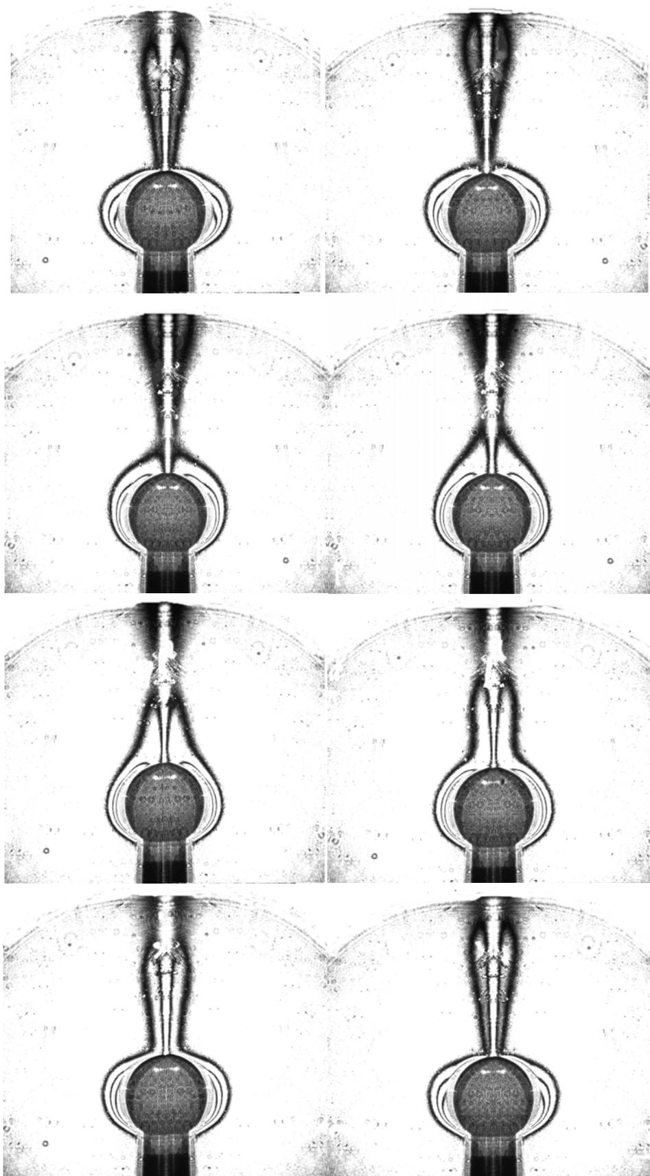
Figure 7. Oscillatory instability of the axisymmetric plume rising from a drop of Methanol dissolved in a Cyclohexane matrix at ambient temperature. The initial volume of the drop is  $5 \mu\text{l}$ . The images are taken at time intervals of 1 seconds.
