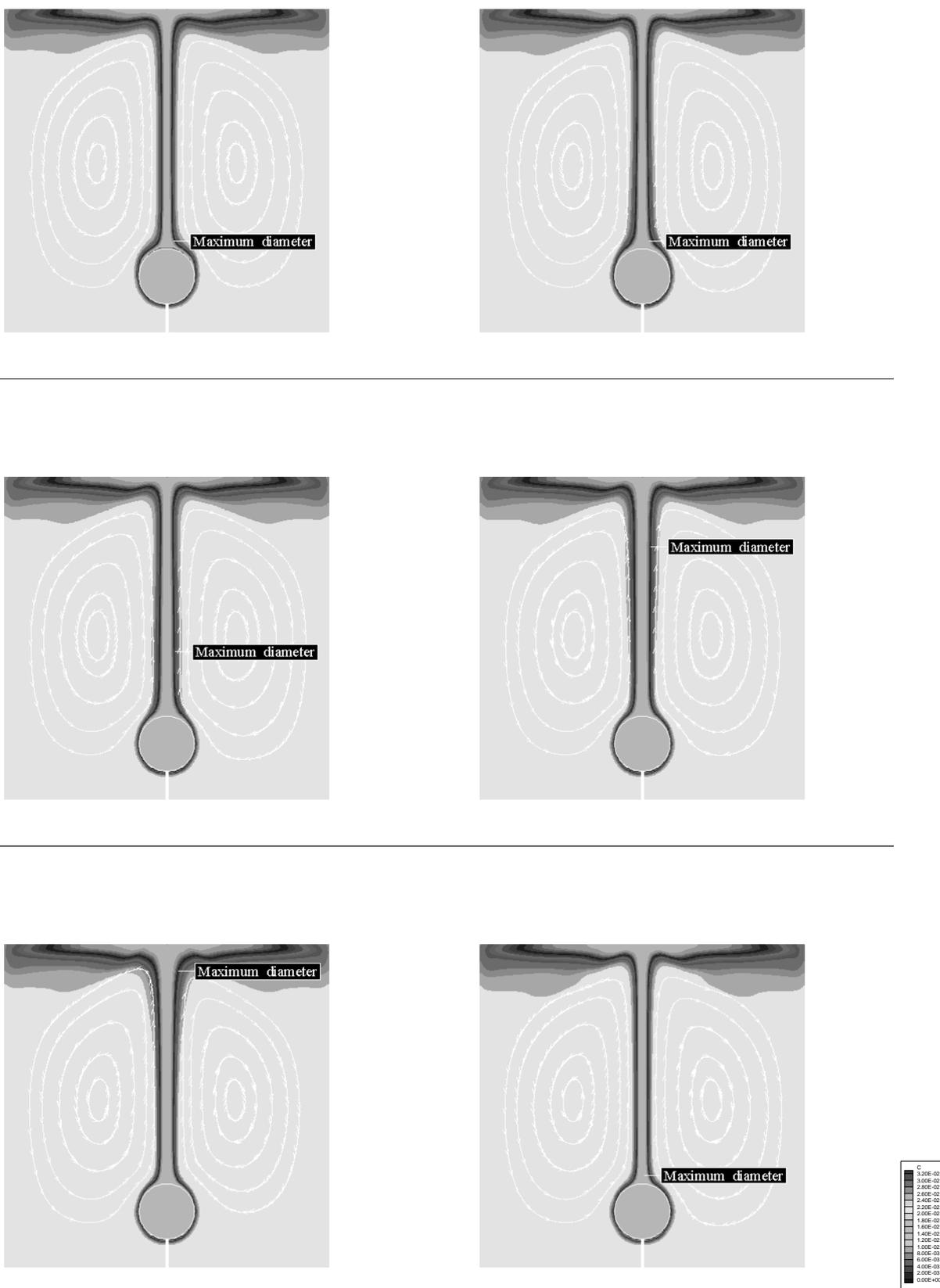
Figure 9. Computed evolution of the unstable solutal plume: concentration and flow field patterns for a 3 [μl] droplet of Methanol dissolving into a matrix of Cyclohexane at ambient temperature ( $V_{max} = 5.4 \cdot 10^{-2}$  [cm/s]).
