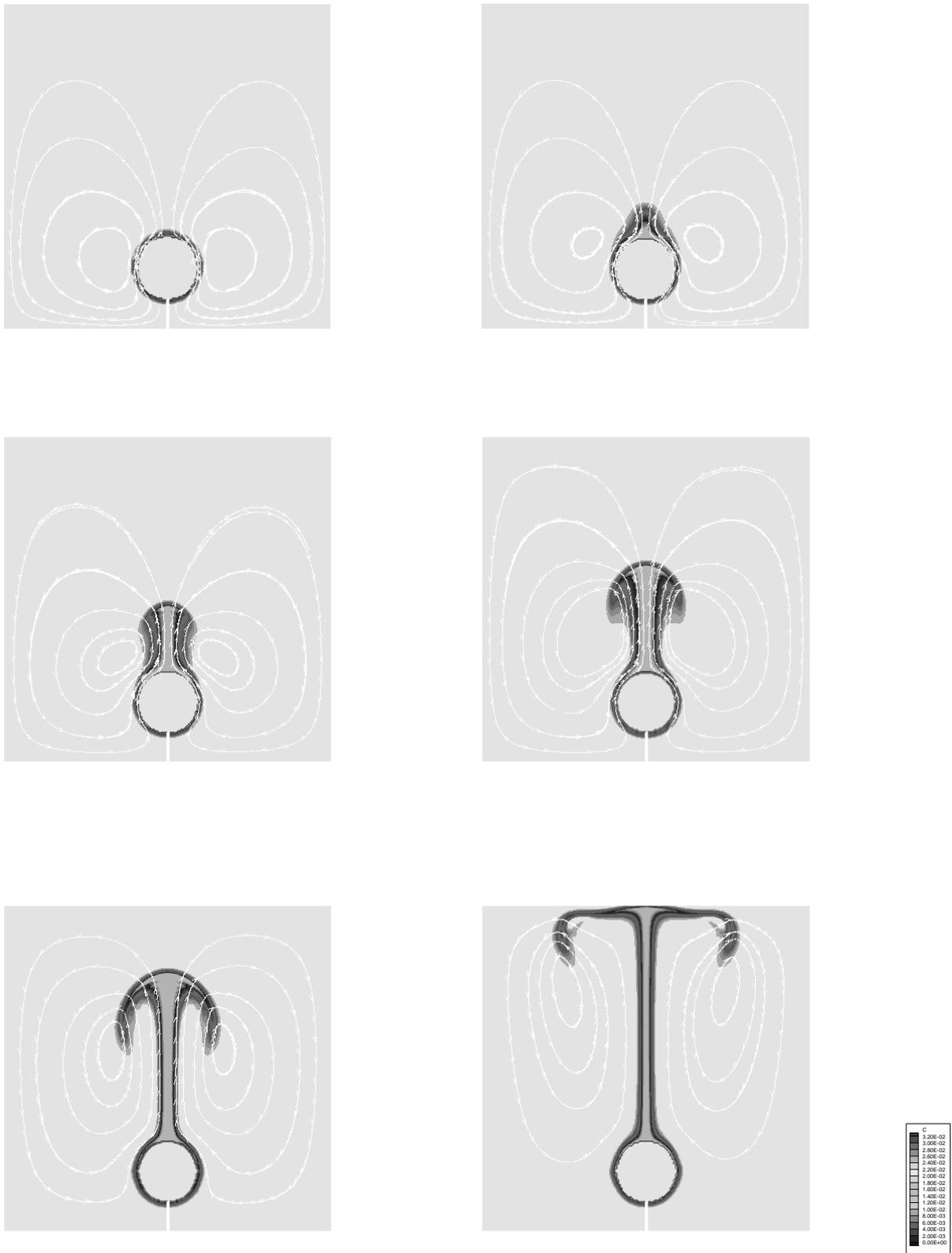
Figure 8. Computed evolution of the concentration and flow field patterns at the beginning of the dissolution process (droplet of Methanol dissolving into a matrix of Cyclohexane at ambient temperature, initial volume of the droplet 3 [ $\mu\text{l}$ ],  $V_{\text{max}} = 5.4 \cdot 10^{-2}$  [cm/s]).
