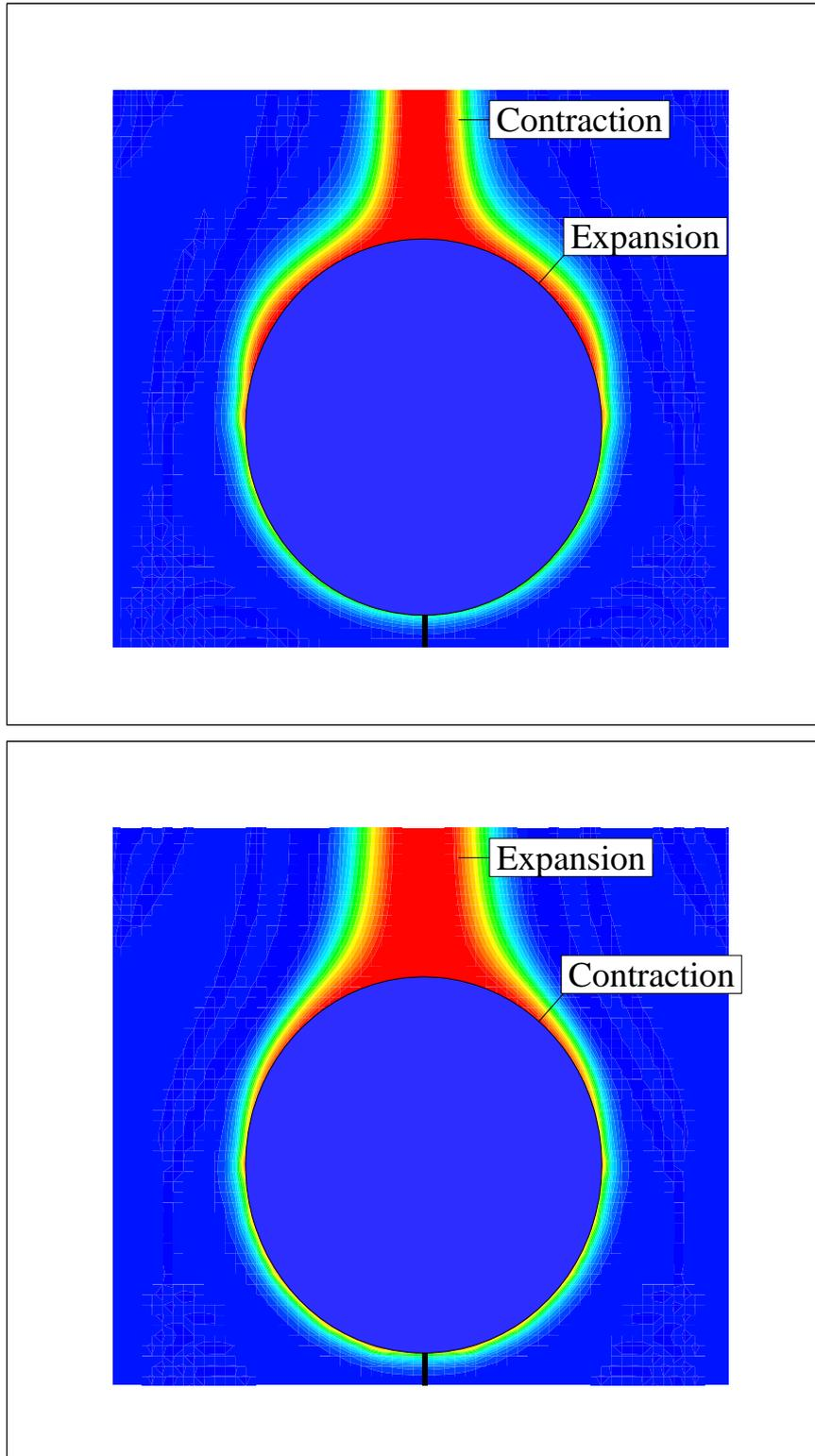
Figure 10. Computed pulsating behaviour close to the surface of the dissolving drop (radial velocity distribution  $V_{\max} = 1.5 \cdot 10^{-2}$  [cm/s]) (Figs (a) and (b) refer to the maximum and to the minimum of an oscillation period respectively)
