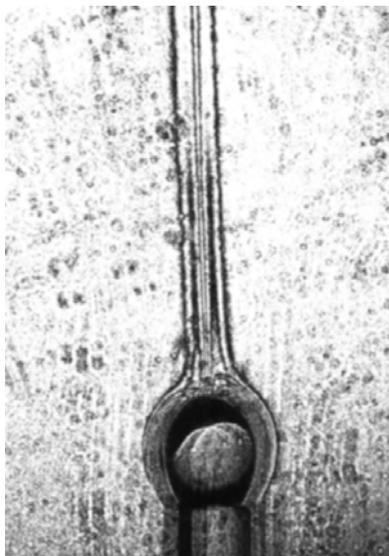
Figure 2. Rising plume from a droplet of Butanol dissolving in water at ambient temperature (initial drop volume of  $1.5 \mu\text{l}$ )
