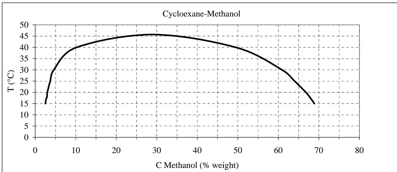
Figure 5. Phase diagram (a) and density versus Methanol concentration (b) for the Cyclohexane-Methanol system
