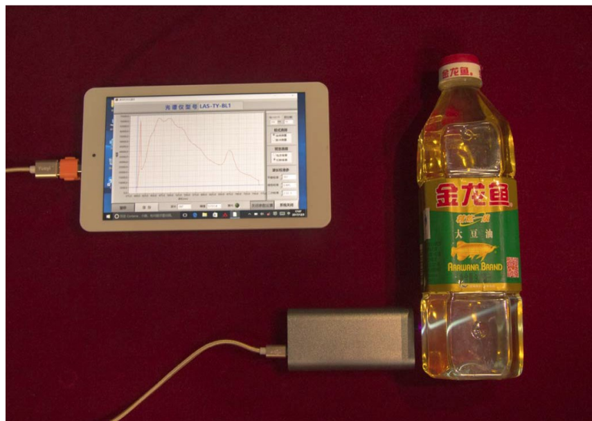
Fig. 2 Picture of testing of edible oil by micro laser fluorescence spectrometer
