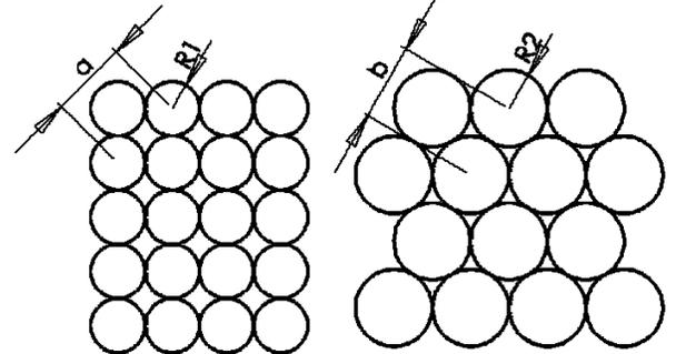
**Figure 1.** Optimal sphere packing (2D case). Left: rectangular packing. Right: Hexagonal (optimal) packing. If we select such  $a, b$ , that  $a=b=\lambda/2$ , then  $R_2 > R_1$ . The same applies for packing corresponding rectangles and hexagons, which fully cover the available area.
