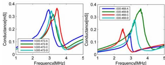
**Figure 11.** Admittance plots of the manufactured devices. Left: Hexagonal element, Right: rectangular element. The typical peak admittance of hexagonal element is higher.
