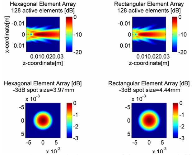
**Figure 4.** Example 2. Comparison of the single-way field generated by a phased arrays comprising equal number of active hexagonal and rectangular elements. The hexagonal-element array produces a tighter focal area.
