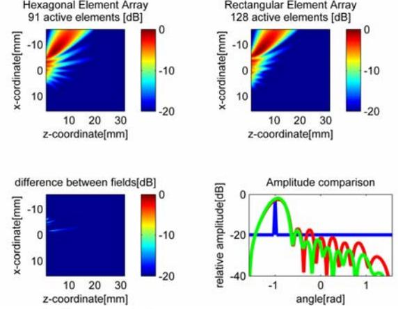
**Figure 3.** Example 1: Simulation of focussed and steered by 1 [rad] acoustic beam. Red –hexagonal-element array; Green – rectangular element array. There are no significant differences between acoustic fields generated.
