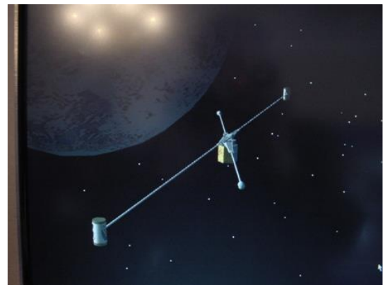
Fig. 1. A motorised momentum exchange tether in LEO.
