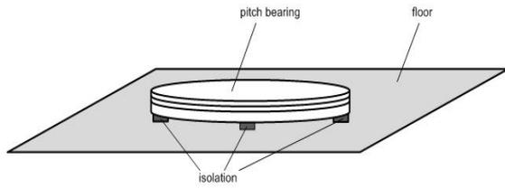
Figure 4. Example of a possible test set-up for a pitch bearing.
