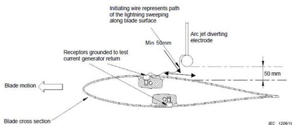
Figure 8. High current (HC) arc entry test.
