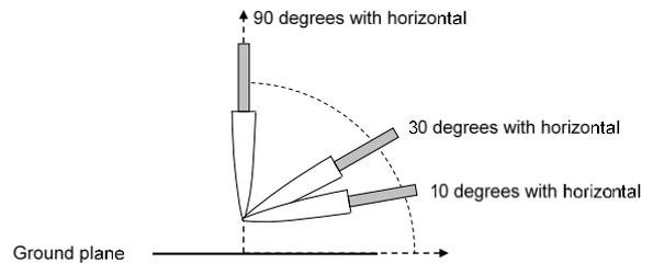
Figure 6. Blade Orientations for initial leader attachment tests.
