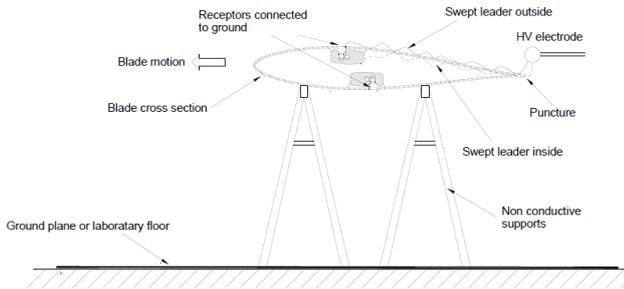
Figure 7. High Voltage (HV) subsequent stroke attachment test.
