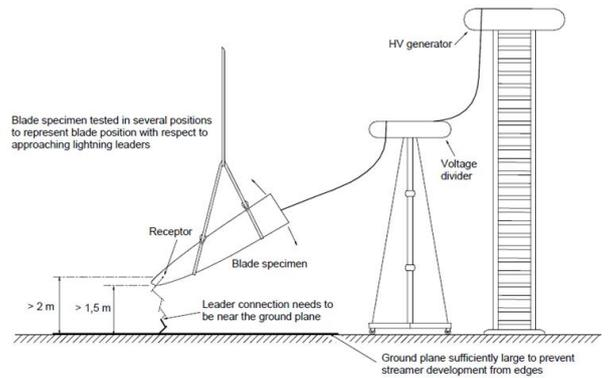
Figure 5. High Voltage (HV) initial leader attachment test.
