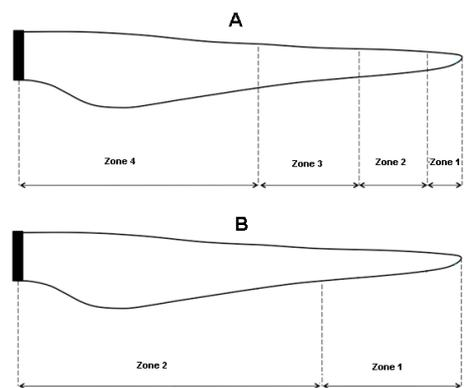
Figure 3. Examples of generic blade lightning environment definition
