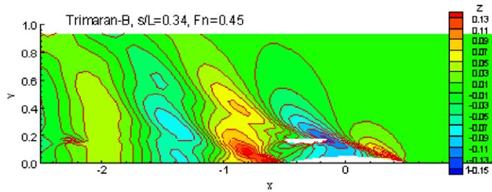
Fig. 11. Wave pattern of trimaran\_B at  $Fn = 0.45$ .
