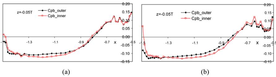
Fig. 9. Pressure distribution on the sub-hull of trimaran\_A for  $s/L = 0.6$ ,  $Fn = 0.30$ ; (a) source/doublet method; (b) source method.
