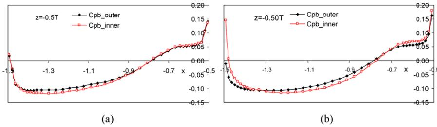
Fig. 8. Pressure distribution on the sub-hull of trimaran\_A for  $s/L = 0.6$ ,  $Fn = 0.30$ ; (a) source/doublet method; (b) source method.
