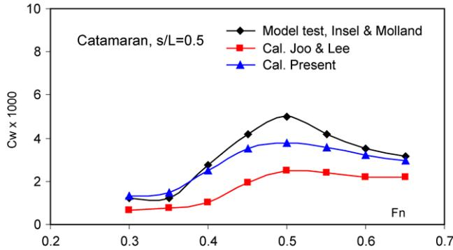
Fig. 3. Comparison of wave-making resistance of a catamaran.
