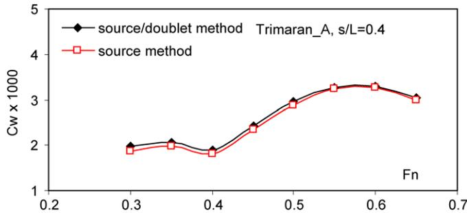
Fig. 6. Wave-making resistance of trimaran\_A.
