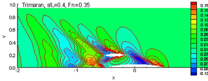
Fig. 5. Wave pattern of trimaran\_A at  $Fn = 0.35$ ,  $s/L = 0.4$ .
