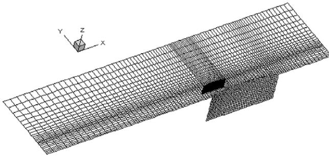
Fig. 4. Panel distribution for a trimaran model.
