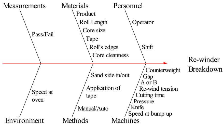
Figure 7. Cause and effect diagram for re-winder
