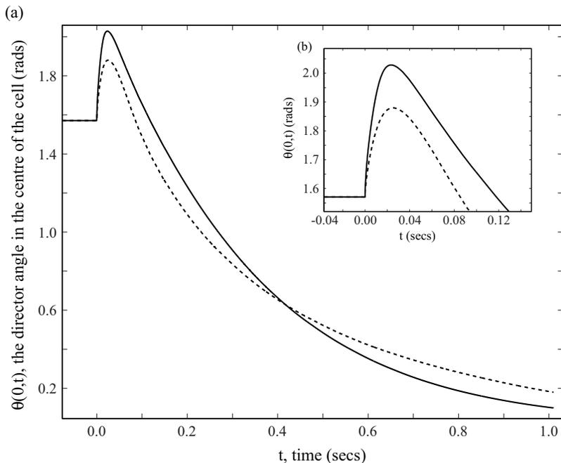
FIG. 1. Comparison between nonlinear (dashed) and linear (solid) solutions: the director angle at the middle of the cell  $\theta(0,t)$  as a function of time. For both cases we have neglected inertia. (b) is a zoomed plot of (a), close to when the magnetic field was turned off.
